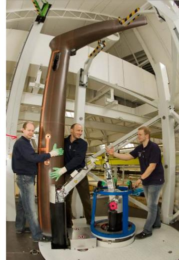
Fig. 9. Preparation of the tail boom inspection at the top platform
