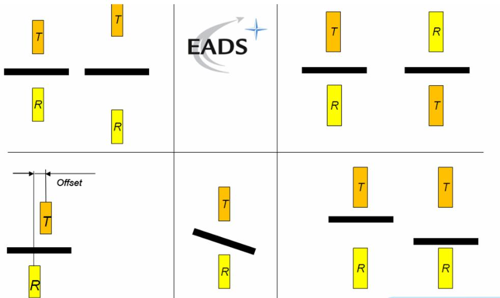
Fig. 6. Study concerning the misfit of the alignment of the probes, T: transmitter, R: receiver transducer
