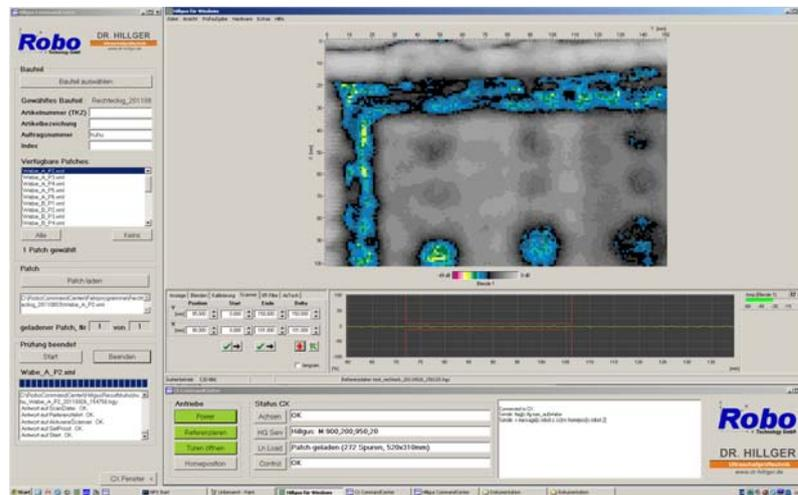
Fig. 10. User interface of the air-coupled ultrasonic system together with the scanner control
