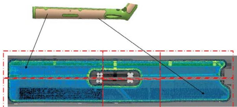
Fig. 11. C-scan of the tail boom
