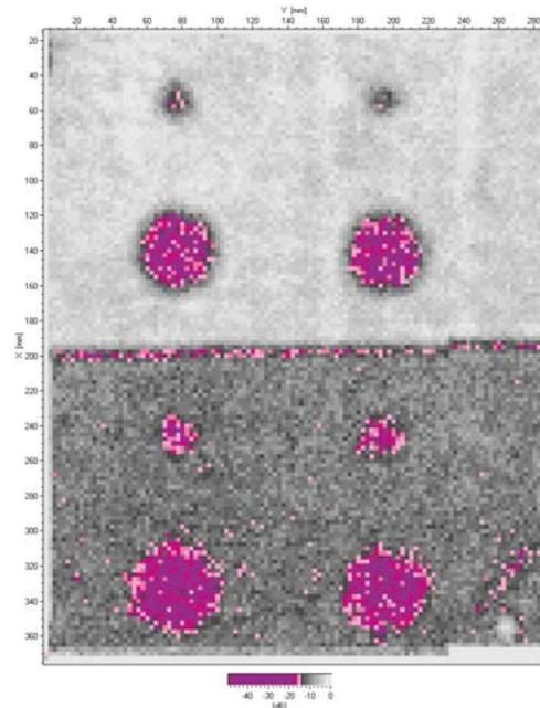
Through-transmission technique with air-coupling
