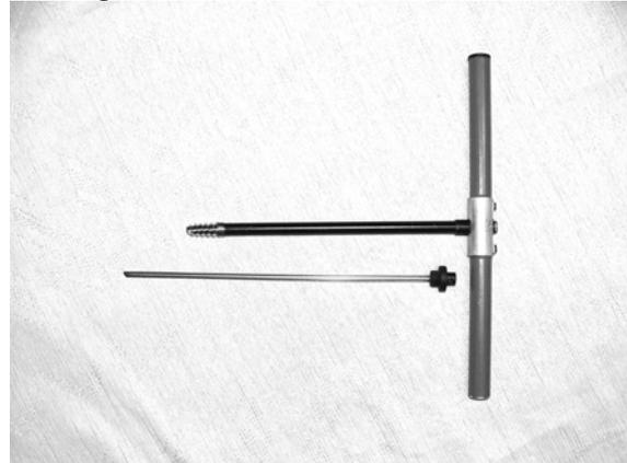
Figure 9. Incremental Wood Drill
