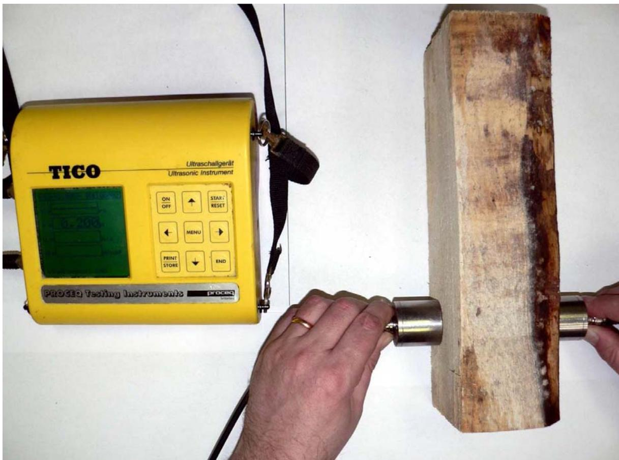
Figure 7. Measurement of Ultrasonic Pulse Transit through a Timber Element – Direct Transmission
