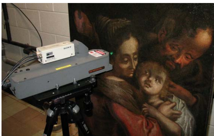
Fig.8 Renishaw® Fiber optic Raman analyzer in operation. University of Windsor, Materials and Surface Science Laboratory.
