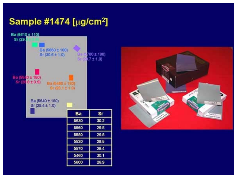
Figure 3. Several experiments were conducted to determine the uniformity of mechanically coated photographic papers.
