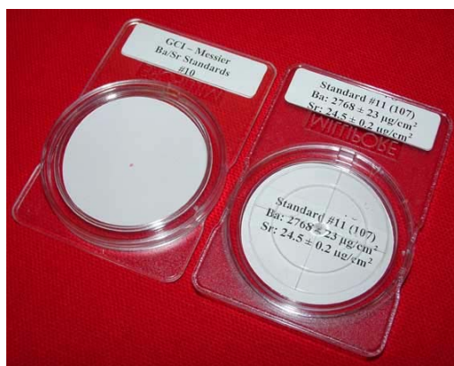
Figure 5. GCI-Messier barium and strontium standards for the quantitative XRF analysis of baryta coated photographic papers.
