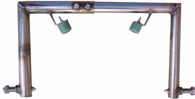
*Fig. 6: The assembly designed to be mounted on the breech of the cannon to install the cathodic protection system: the stainless steel structure, the insulated pressure caps and the metallic tips (insulated from the arch) for electrical connection with the cast-iron under the graphitization layer can be observed.*
