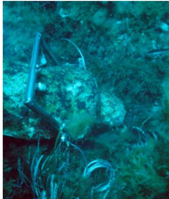
*Fig. 7: Photographs of the cannon laying on the seabed after CP system installation: a) potential measurement by Corrintec; b) detail of the arch and the connected anode wires (photos ICR).*
