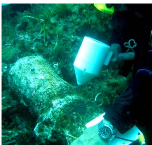
*Fig. 4: Corrosion potential measurement by Corrintec Rust Reader (Photo ICR)*
