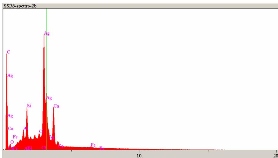
Fig.6: SS8 EDX spectrum of black area
