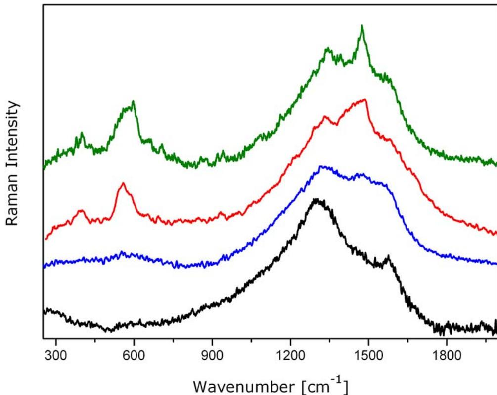
Figure 6: Raman spectra of original inks compared to standards. MS Piana 3.207 (blue line); Arabic ink (red line); carbon black (black line); iron-gall ink (green line).
