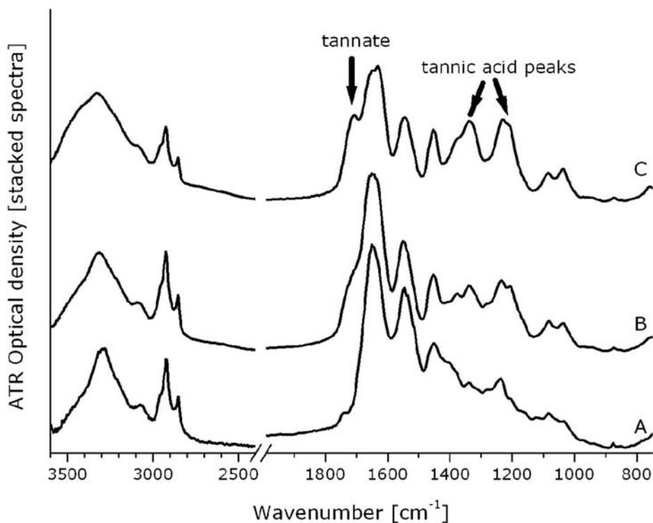
Figure 2: ATR/FTIR spectra of parchment samples -hair sides- after removal of  $\text{CaCO}_3$  (spectrum A), after removal of  $\text{CaCO}_3$  and addition of tannic acid 2 g/l (spectrum B), after removal of  $\text{CaCO}_3$  and addition of tannic acid 10 g/l (spectrum C).
