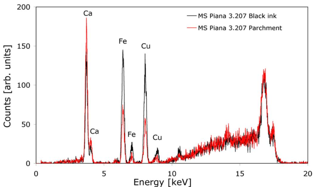
Figure 7: XRF spectra of MS Piana 3.207. Black line: ink; red line: parchment.
