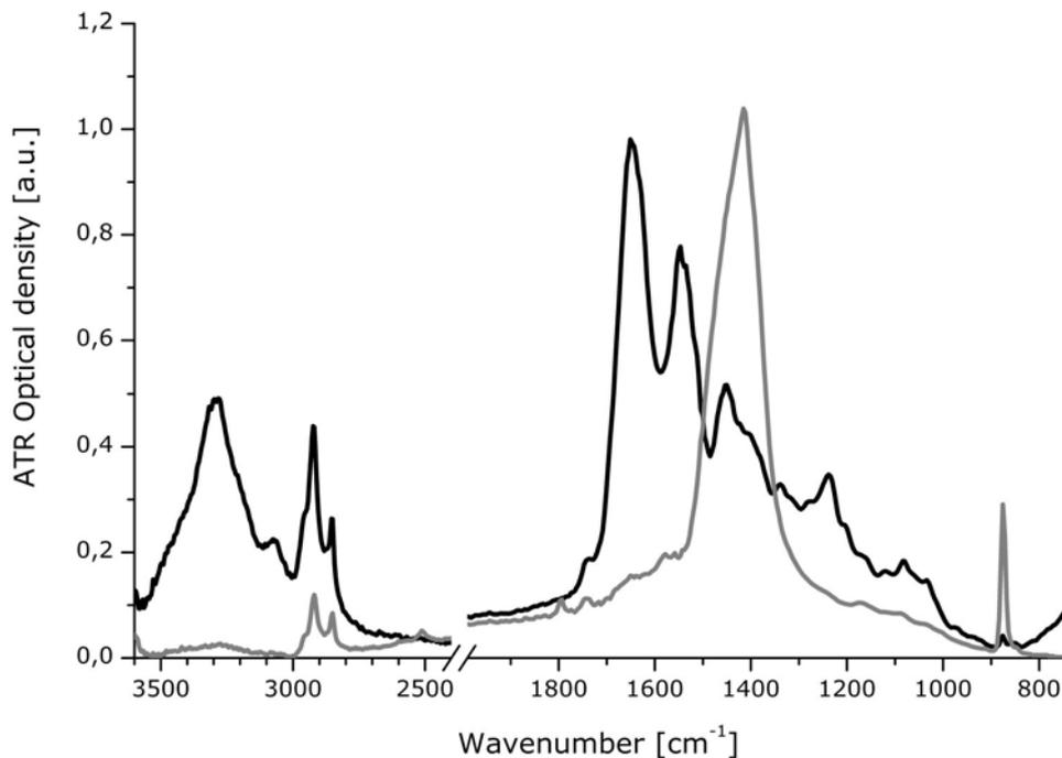
Figure 1: ATR/FTIR spectra of parchment samples prepared in laboratory. Untreated (grey) and after removal of  $\text{CaCO}_3$  (black)
