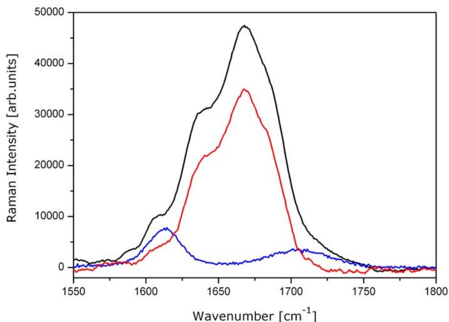
Figure 3: Raman spectra of parchment samples -hair sides- after removal of  $\text{CaCO}_3$  (red line), after removal of  $\text{CaCO}_3$  and addition of tannic acid 10 g/l (black line) compared to tannic acid (blue line).
