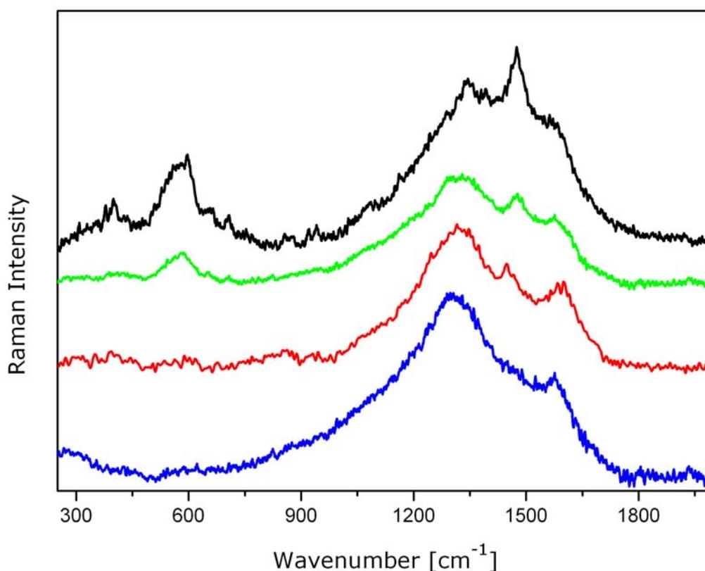
Figure 5: Raman spectra (stacked) of different inks on the laboratory samples. Carbon black (blue line); carbon black with iron II sulfate (red line); carbon black with iron-gall ink (green line); iron-gall ink (black line).
