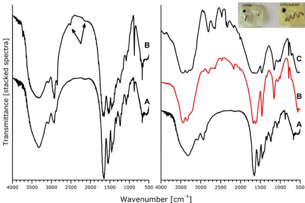
Figure 9. Left: FTIR spectra in KBr of an intact (A) and a burned (B) parchment. Right: FTIR spectra of parchment treated with urea (B) and reference materials, pure urea (C) and untreated parchment (A).
