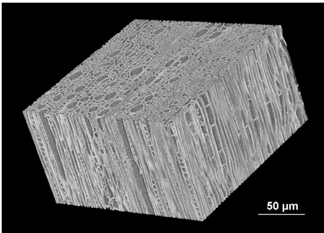
*Figure 4 – Three dimensional rendering of a sample of Quercus caducifolia impregnated with isoeugenol polymerized, obtained by SR-CT.*
