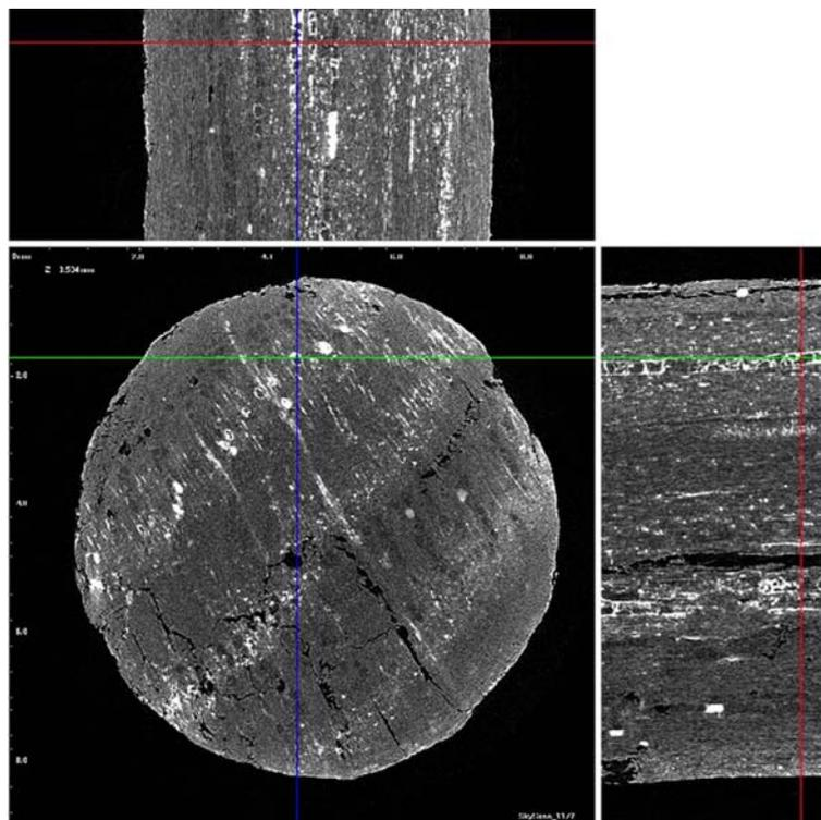
Figure 1 – Cross section of a sample of *Quercus caducifolia* impregnated with a mixture of PEG 1500 at 20% in PPG 425, obtained by  $\mu$ -CT
