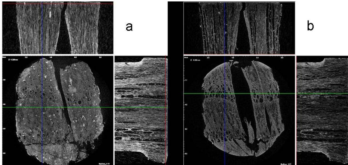
Figure 2 – Cross sections of a sample of *Quercus caducifolia* impregnated with isoeugenol polymerized *in situ*, obtained by  $\mu$ -CT: (a) surface; (b) 4.5 mm from the surface
