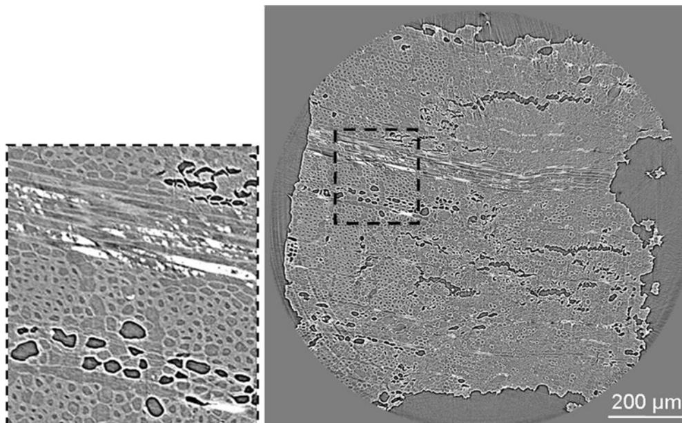
Figure 3 - Cross section of a sample of *Quercus caducifolia* impregnated with a mixture of PEG 1500 at 20% in PPG 425, obtained by SR-CT.
