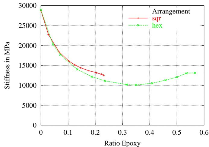
Figure 8: Stiffness of square and hexagonal unit cells after variation of aspect ratio
