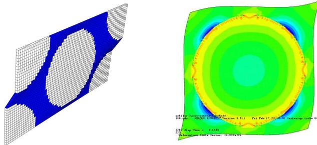
Figure 5: Deformations caused by in-plane shear (left) and transverse shear (right)
