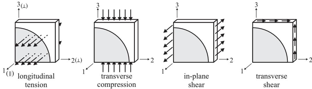
Figure 4: Different loading conditions
