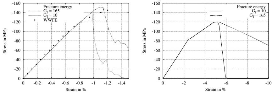
Figure 9: Influence of fracture energy on unit cell (left) and matrix material behavior (right)
