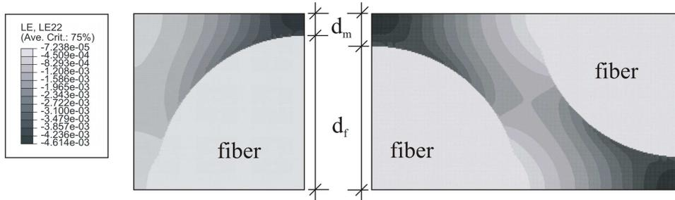
Figure 7: Strain distribution in square and hexagonal arrangement of unit cell
