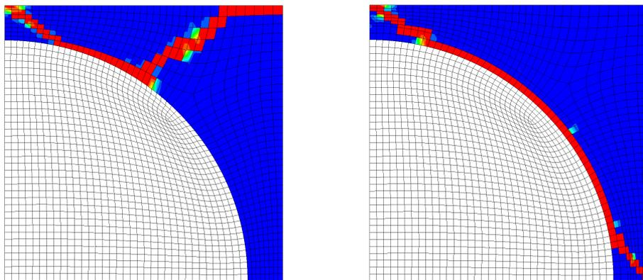
Figure 10: Damage evolution in conventional mesh dependent on mesh
