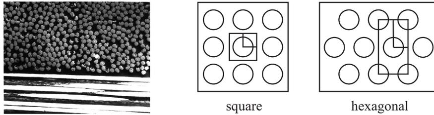
Figure 2: Micrograph (left) and assumed arrangement of fibres for unit cells
