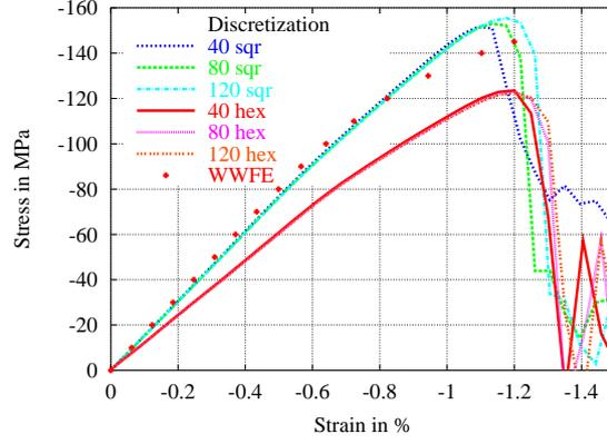
Figure 6: Stress-strain curves for different discretizations under transverse compressive strain compared to test results from WWFE
