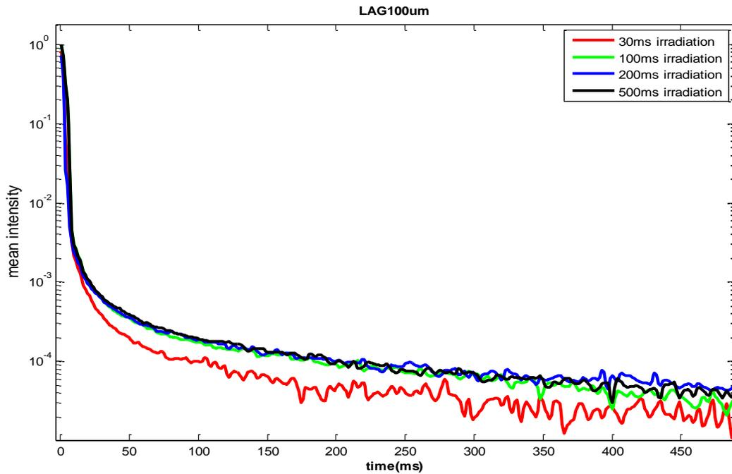
Figure 4: Afterglow for different amounts of irradiation using LAG100um
