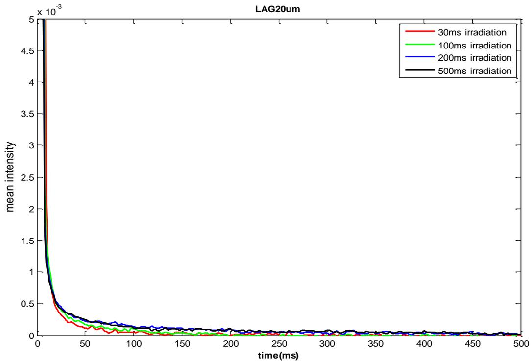
Figure 5: Afterglow for different amounts of irradiation using LAG20um
