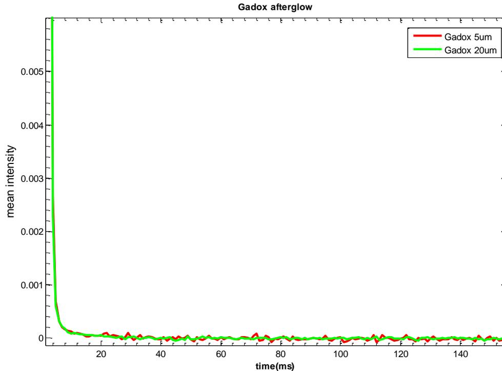
Figure 7: Afterglow of two different thickness of Gadox scintillator
