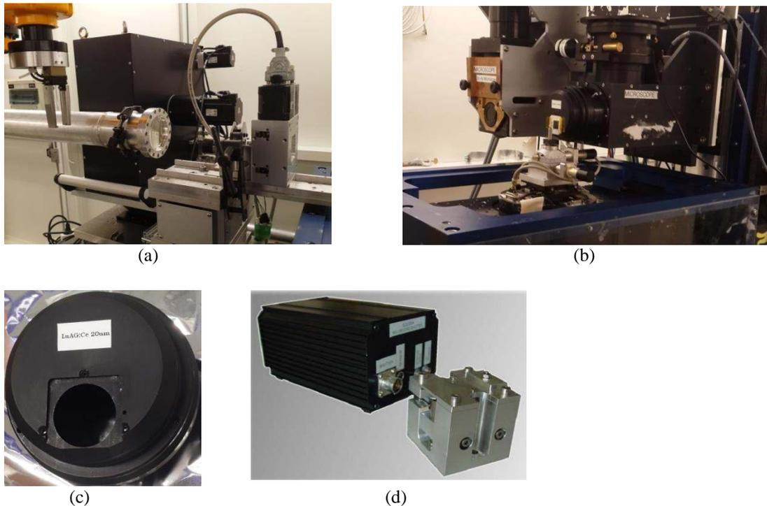
Figure 1 Experimental setup at the TOMCAT beamline. (a) The beamline vacuum fly tube and beam conditioning tower with the SLS 2004 Millisecond Shutter and a slit system. (b) Two different microscope optics with scintillators (c) Close-up view of the mounting place for the scintillator. (d) SLS 2004 Millisecond Shutter and its control unit.
