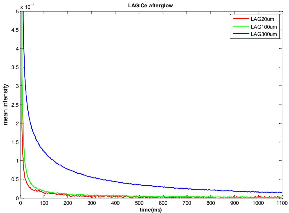
Figure 6: Afterglow of different thickness of LAG scintillator
