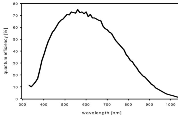
Figure 2: (a) pco.EDGE 4.2 with sCMOS sensor. (b) Quantum efficiency of pco.EDGE 4.2 (~70% at 535 nm)
