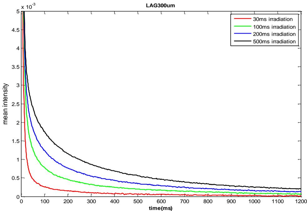
Figure 3: (a) Afterglow for different amounts of irradiation using LAG300um
