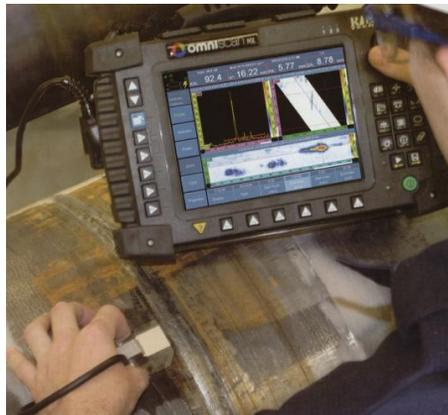
The critical aspect of qualification is detection of all pertinent flaws. ASME has provided for a generic sensitivity and angle beam coverage in Section V requirements for manual ultrasonic testing. Carrying out ultrasonic inspections to these guidelines precludes any need to qualify the techniques. However, the detection of all pertinent flaws over the required reference level at the required sensitivity need not always occur when following the
