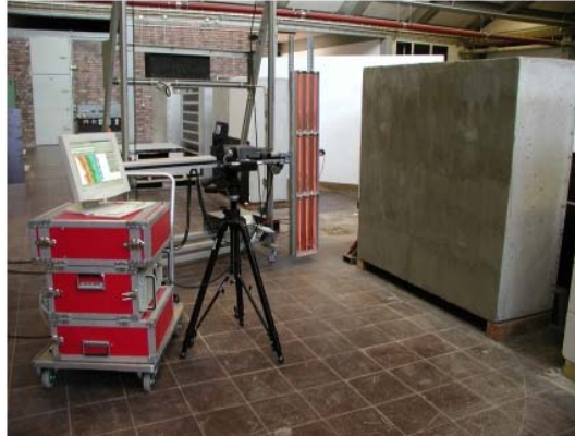
Figure 3: Experimental set-up for laboratory investigations at BAM with investigated specimen A.
