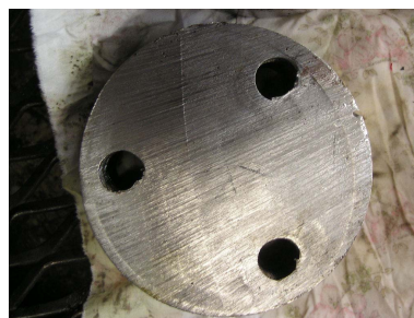
Fig. 16. Forged impurities at axle beginning.
