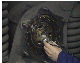
Figure 10: Probe positioning at axle front face.
