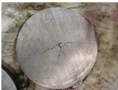
Fig. 15. Forged impurities close to axle centre.
