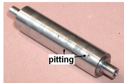
Fig.3 R-mat device (a) and test sample with pitting in traces (b).
