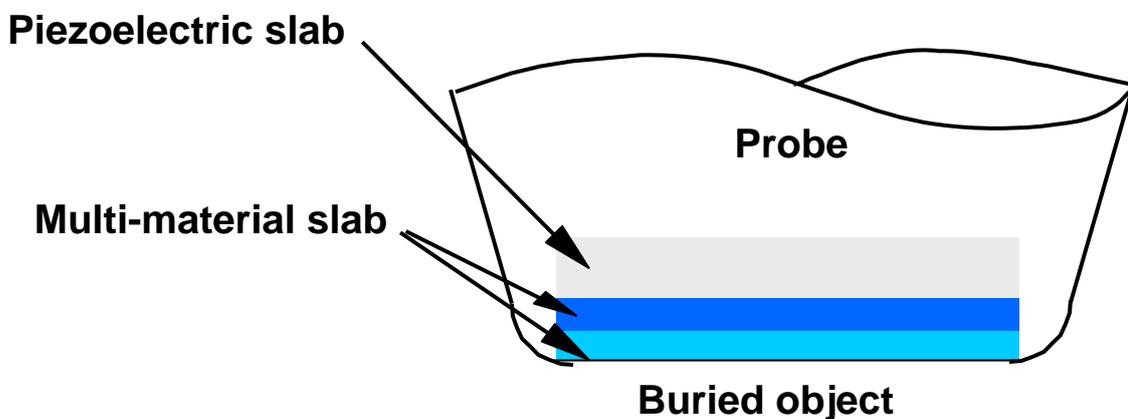
**Fig. 2.** Sketch of a multi-layer tip of a hand probe.
