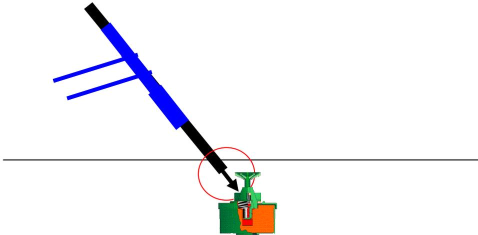
**Fig. 1.** Sketch of a working principle of a hand probe with integrated ultrasonic sensor. Blue – automated system for hand probe manipulation, black – hand probe, red circle – area of functioning of an ultrasonic sensor mounted near the hand probe tip.
