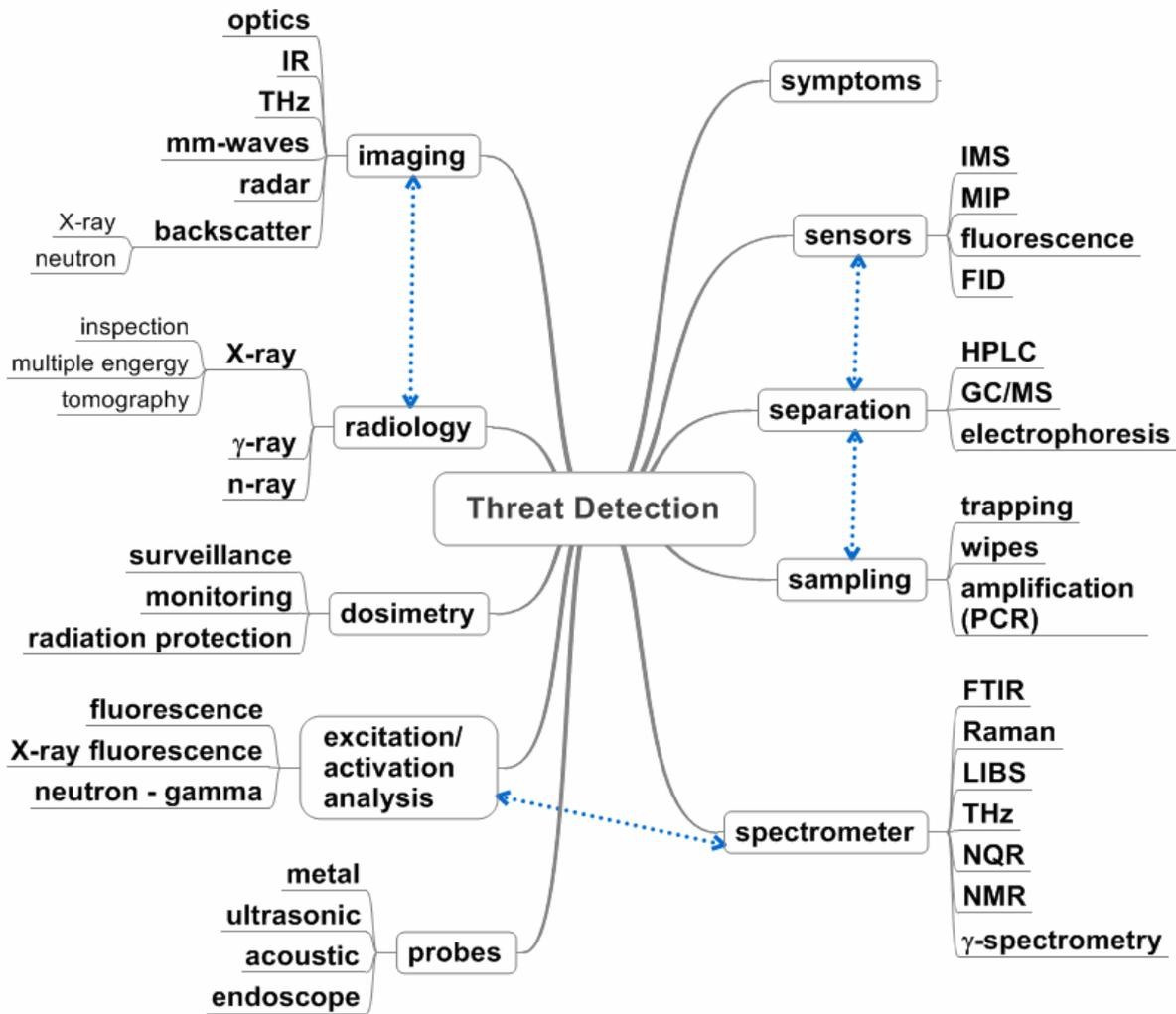
Fig. 5: An overview of threat detection technologies
