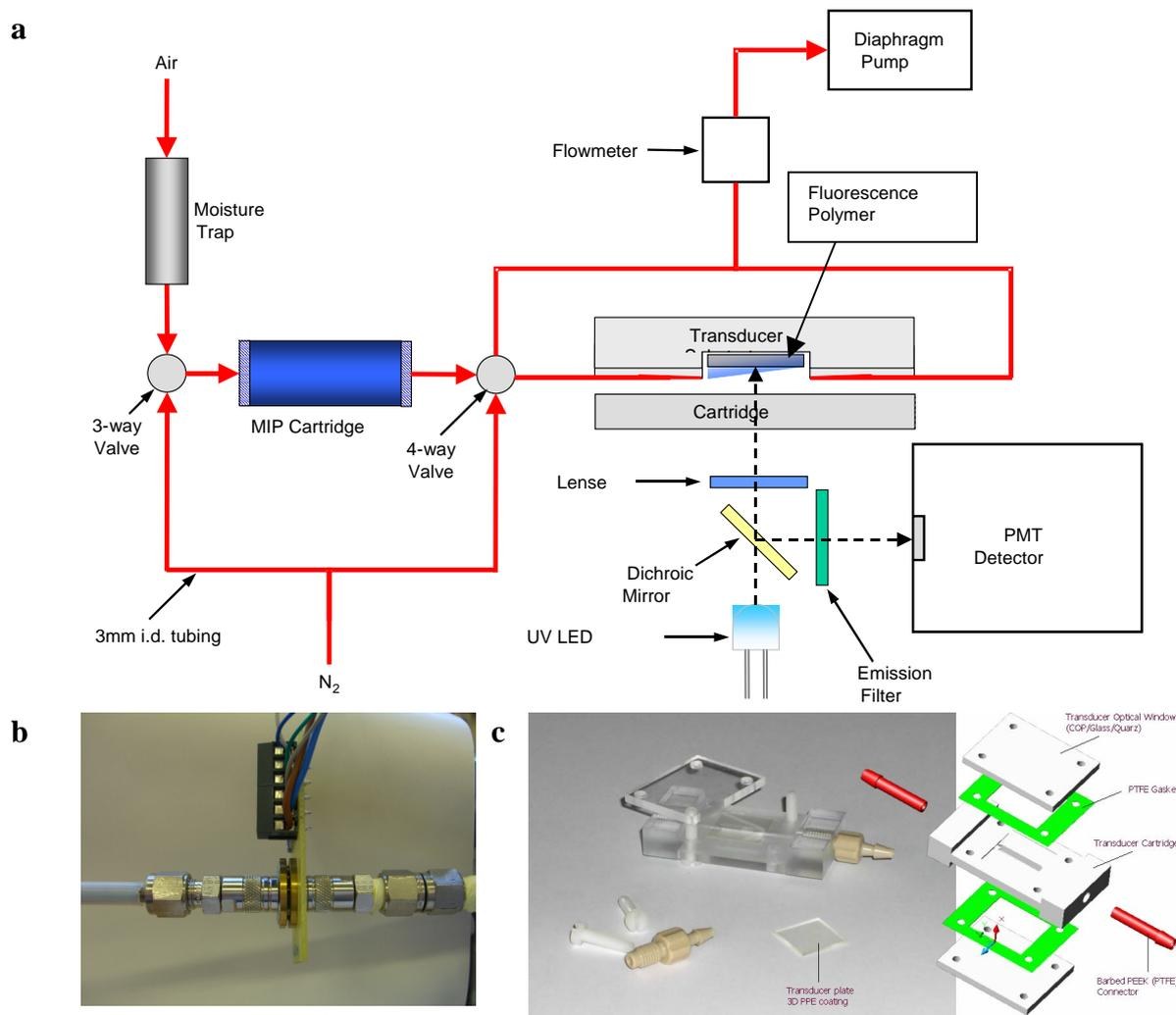
Fig. 6: TNT chemosensor device: Functional diagram with molecular imprinted polymer (MIP) and transducer module as functional components, gas flow and optical unit (a), MIP cartridge (b) and transducer (c).
