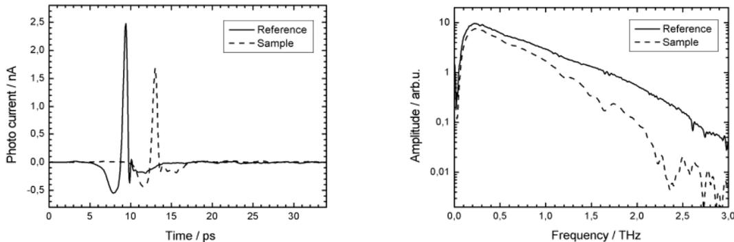
**Figure 2.** THz waveforms (a) measured with a sample (dashed) and without any sample (solid) placed in the spectrometer. The corresponding frequency amplitude spectra (b) obtained by Fourier transform algorithm (FFT) yield information about the transmission characteristics of the sample.
