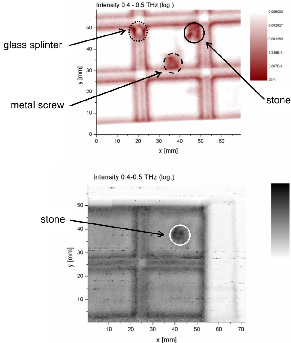
**Figure 5.** THz images of two artificially contaminated chocolate bars: a stone (solid circle), a M2 metal screw (dashed circle) and a glass splinter (dotted circle). Below: Another chocolate bar contaminated with a stone in its original plastic package.
