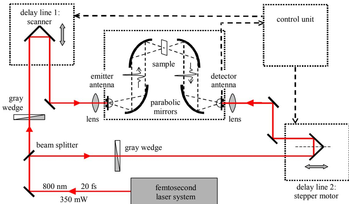
**Figure 1.** Schematic of the applied THz time-domain spectrometer.
