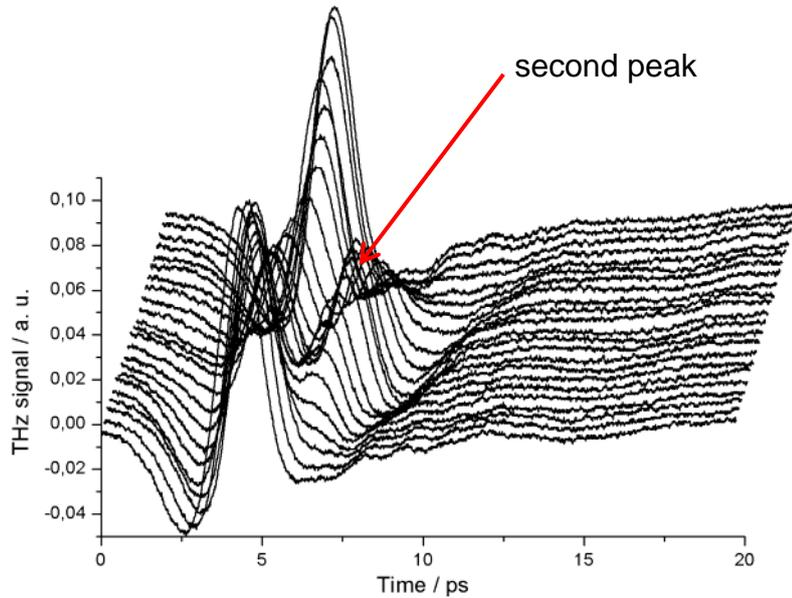
**Figure 6.** Waterfall plot of THz waveforms measured moving the chocolate bar with a glass splinter step by step across the THz beam.
