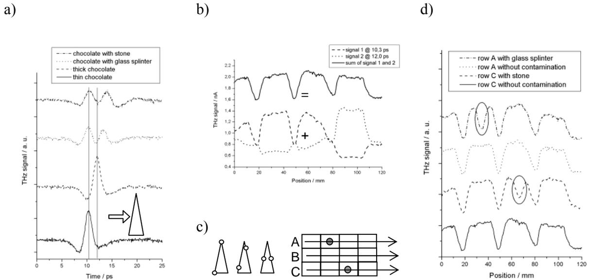
**Figure 7.** a) THz waveforms through pieces of chocolate with and without contamination, b) adding two line scans, c) approximation of the THz pulse with a triangle, schematic of a chocolate bar with contaminations d) sum of line scans through rows with and without contamination
