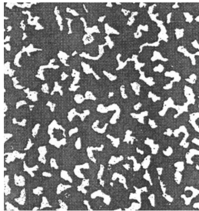
Fig. 3. Ferrite-pearlite structure related to the number 4
