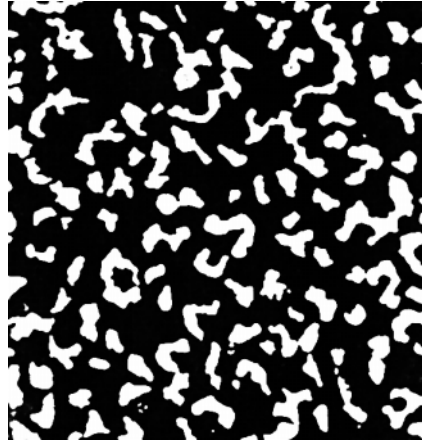
Fig. 5. The image of ferrite-pearlite structure (scale number 4) after processing
