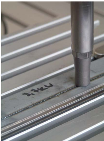
Fig. 1: Eddy current probe on laser welding seam
