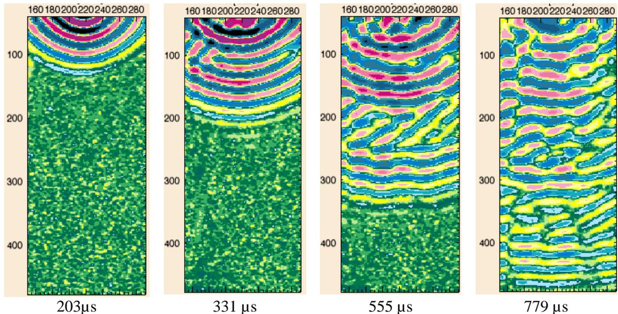
Fig. 5: Lamb wave propagation in sandwich specimen 1.2.3 (impacted with energy of 15 J)
