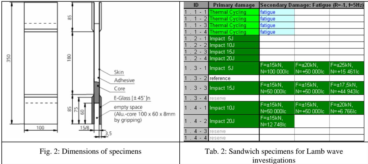
Table 2 presents an overview of the honeycomb specimens. For each type of specimen there remains one reference sample without loading. This is important for the optimisation of the test parameter for Lamb waves. The table also gives information on the type of loading such as thermal cycling (degradation), impact and fatigue.
