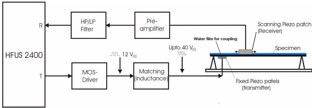
Fig. 4: Experimental setup for wave visualisation with direct coupling
