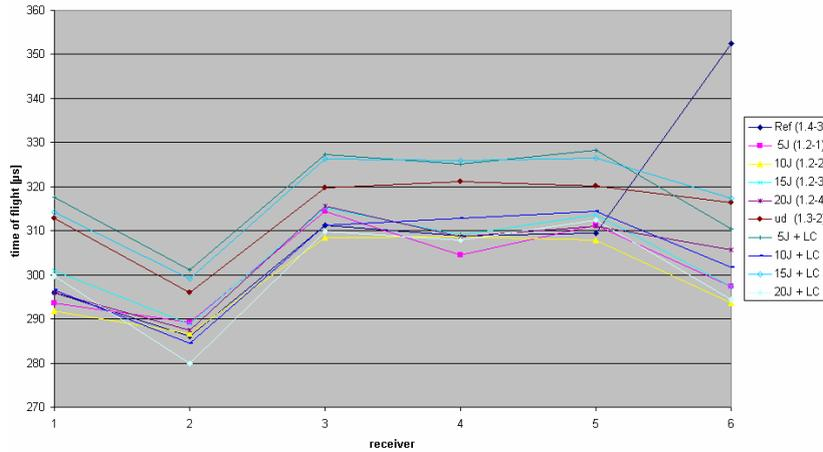
Fig. 2: Time of flight at six positions of sandwich specimens with different loadings
