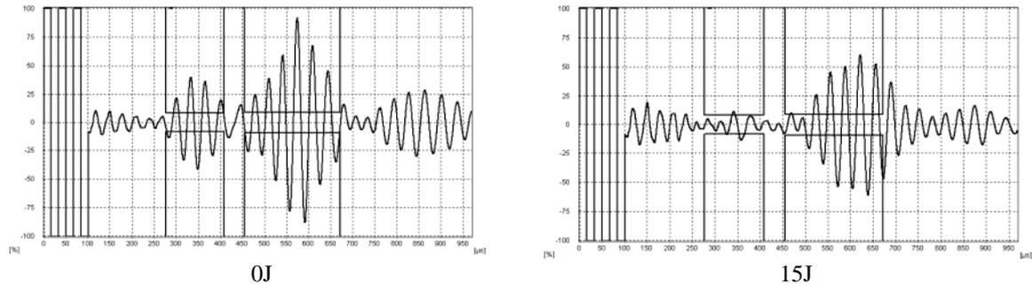
Fig. 6: Lamb wave A-scans received from sandwich specimens without impact and with a 15 J impact
