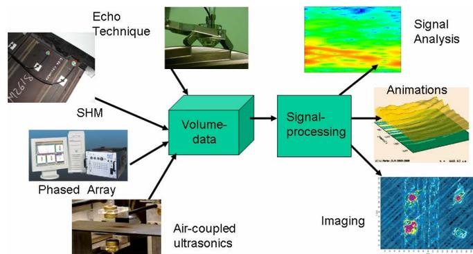
Fig. 3: Network of different NDT-methods
