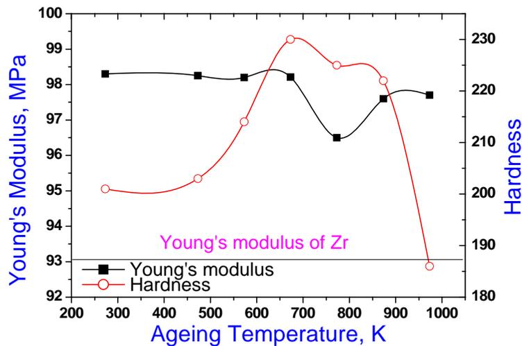
**Fig. 3.** Variations in Young's modulus and hardness with ageing temperature in Zircoloy-2. Young's modulus of pure zirconium is also shown for direct comparison.
