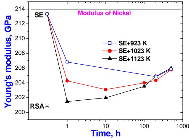
**Fig. 1.** Variation in Young's modulus with post service thermal ageing in Inconel 625 (SE-service exposure and RSA- re-resolution annealed). Modulus of pure nickel is also shown for direct comparison.
