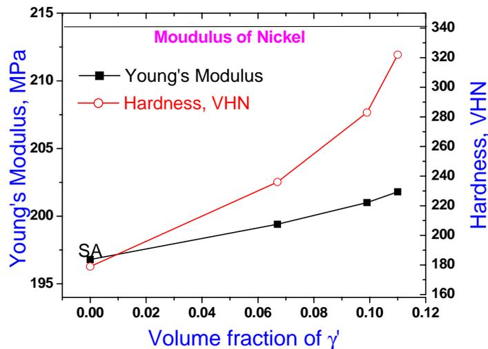
**Fig. 2.** Variation in Young's modulus with volume fraction of  $\gamma'$  in Nimonic PE 16. Modulus of pure nickel is also shown for direct comparison.
