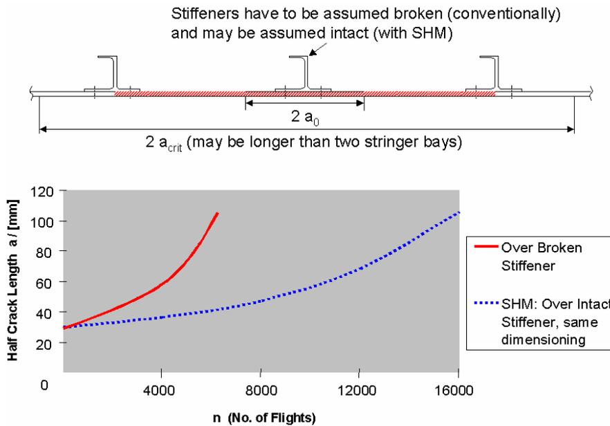
**Figure 2:** Example for assumed crack growth on fuselage structure, conventionally inspected and with SHM
