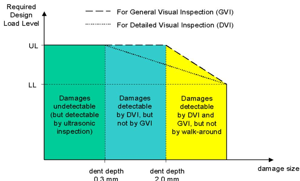
Figure 3: Required design load level versus detectable damage size.
