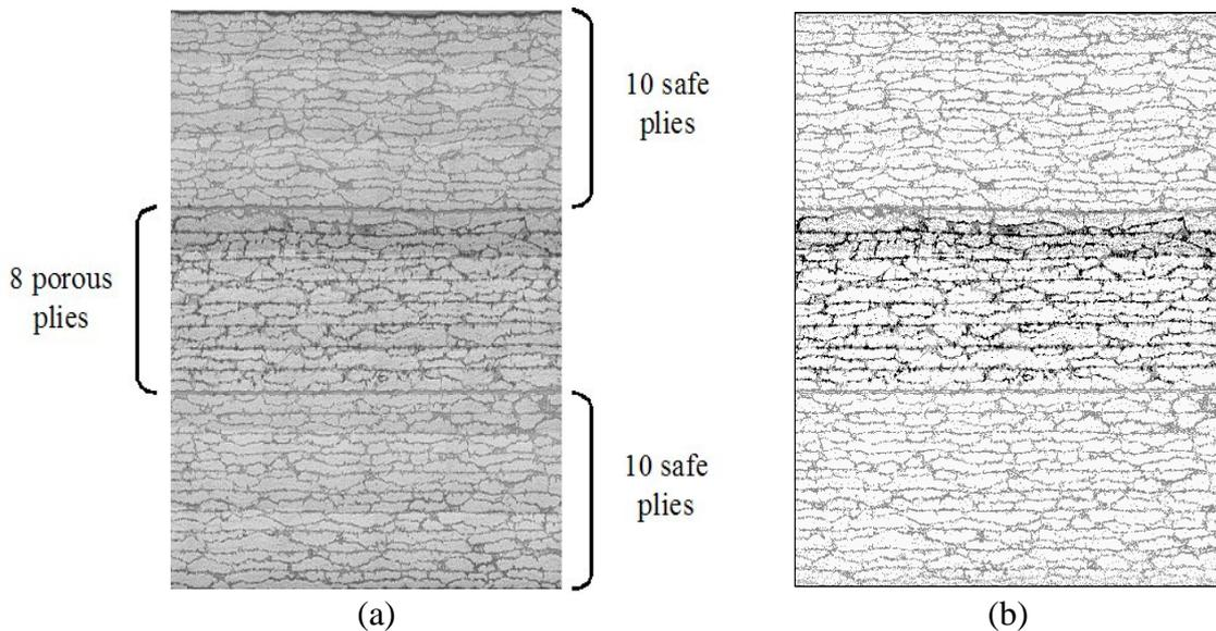
**FIGURE 3.** (a) Microphotograph of a carbon-epoxy material with a localised porous zone (8 central plies), (b) Propagation medium for the modelling.
