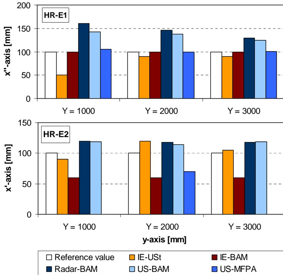
Fig. 3: Localising tendon duct (HR-E1 and HR-E2), relating to relative coordinate  $x^I$  and  $x^{II}$
