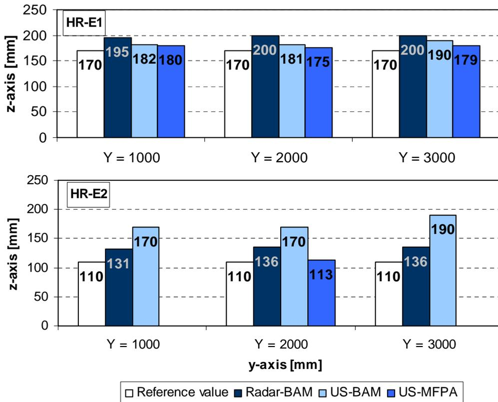
Fig. 4: Concrete cover of tendon duct (HR-E1 and HR-E2)
