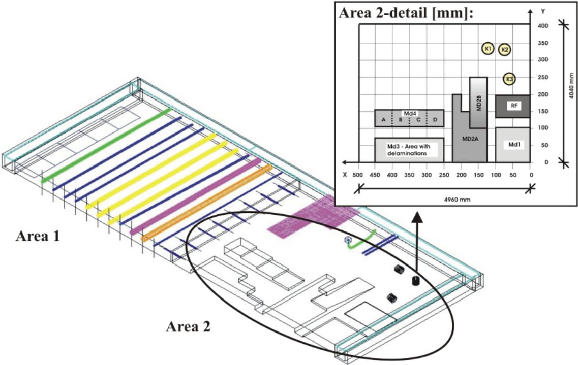
**Fig. 1:** Drawing of the large concrete specimen (LCS) at BAM with details of area 2 (part with artificial flaws), dimensions in mm
