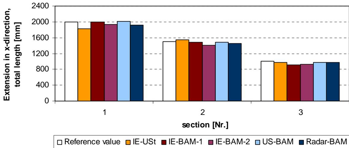
**Fig. 2:** Extensions (section 1-3) in x-direction of a measured flaw
