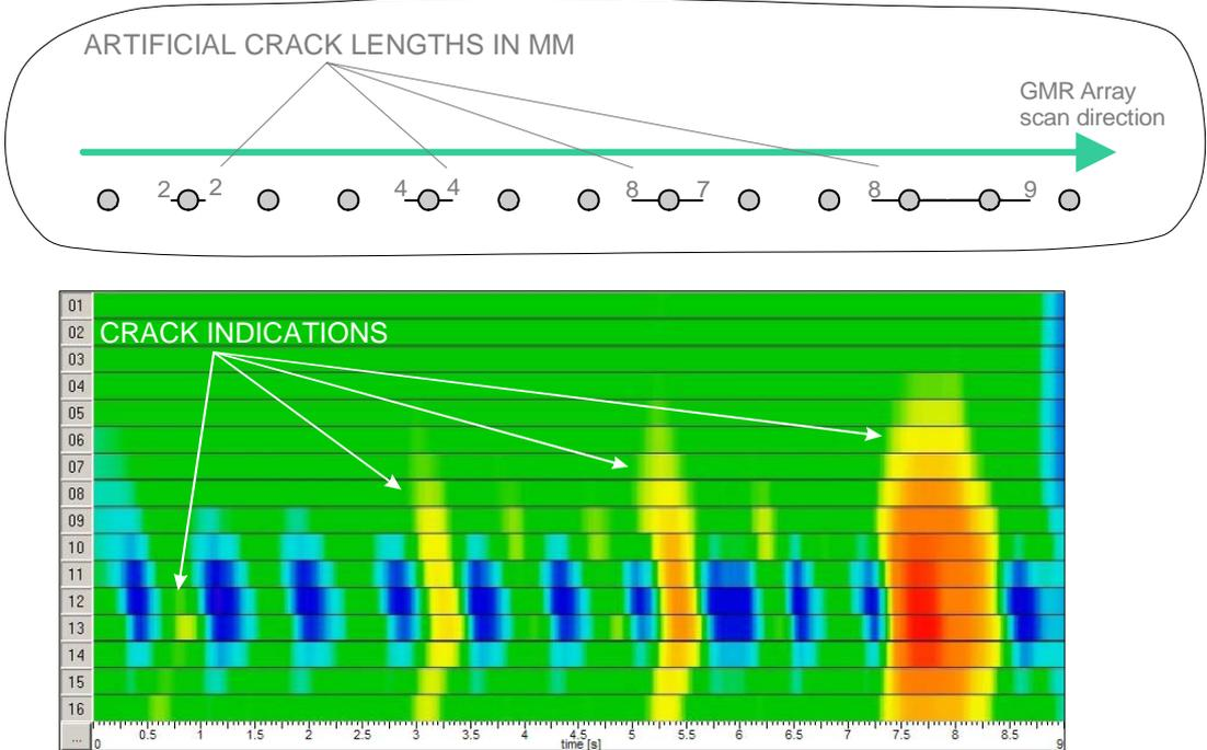
**Figure 6:** Layout of the lap joint of aluminium panels with artificial hidden defects (on the top) and the corresponding result of the measurement with the GMR sensor array (colour-coded C-scan image, on the bottom)
