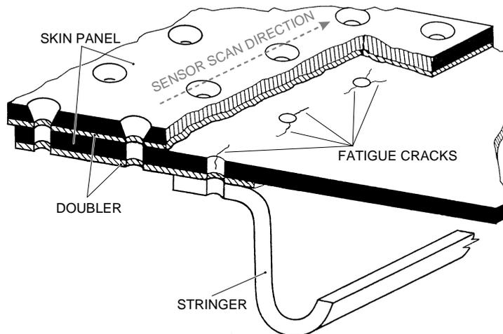
**Figure 5:** Longitudinal lap joint with fatigue cracks in an aircraft skin panel (typical example)
