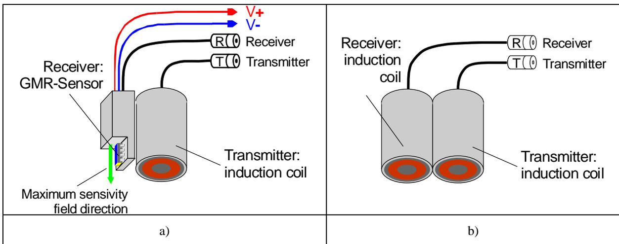
**Figure 1:** Basic arrangements of EC GMR probe (a) and a comparable inductive EC probe - so called half-transmission probe (b).
