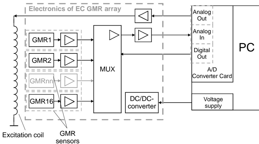
**Figure 3:** Block diagram of the inspection system with EC GMR array
