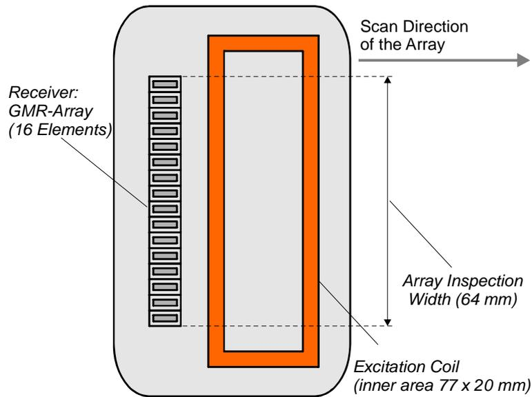
**Figure 2:** Arrangement and main dimensions of the EC GMR Array
