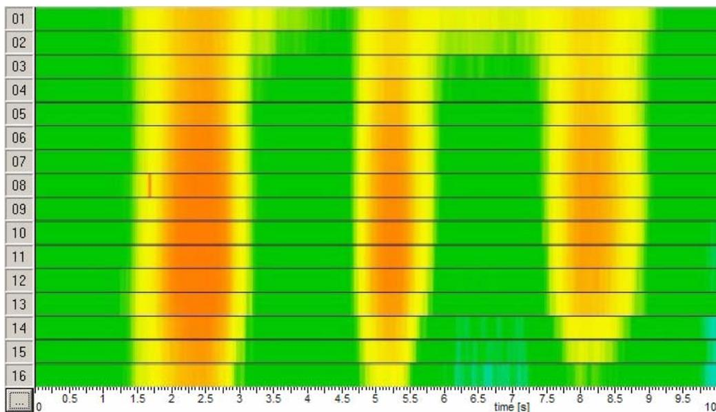
**Figure 8:** Investigation of the maximal inspection depth in aluminium: Result of the measurement with the GMR sensor array (colour-coded C-scan image), obtained on the specimen according to the fig. 7. EC frequency 100 Hz; Cover depth: 20.4 mm
