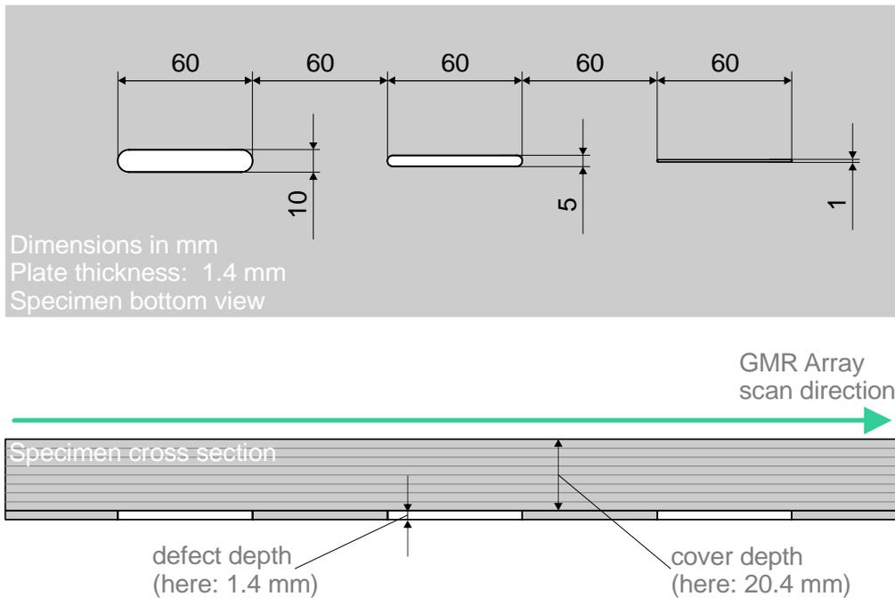
**Figure 7:** Investigation of the maximal inspection depth in aluminium: Geometry of the specimen with fixed depth of the hidden defect and the variable cover depth
