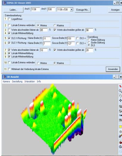
**Figure 6.** Screenshot of the user-interface of the postprocessing and 3D-imaging system.
