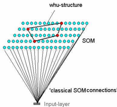
**Figure 4.** Schematic SOM with a Whu-structure
