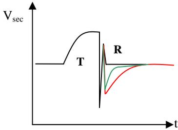
**Figure 1.** Schematic representation of the time-dependent decay of induced pulse with cases black: no metal, red: good and green: poor conductor. T denotes the transmission phase, R denotes the receiving phase.
