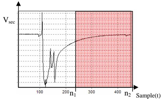
**Figure 2.** Example for the use of a fixed sized integration window to generate the acoustic signal to denote the metal content by a TDM detector (shown is a real signal received when moving the sensor head over a mine with “high” metal content).
