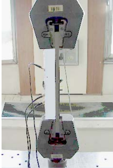
Fig. 4: Tensile test on test-tube taken in the base metal or the melted zone
