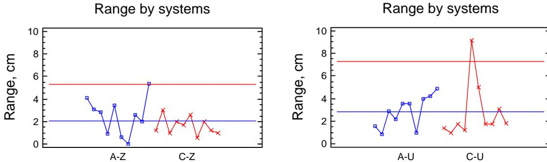
**Figure 2.** Ranges of pinpointing results (3 repetitions) for each of 10 targets obtained by **operators A and C** using **devices Z and U**.
