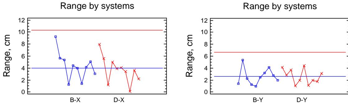
**Figure 3.** Ranges of pinpointing results (3 repetitions) for each of 10 targets obtained by **operators B and D** using **devices X and Y**.
