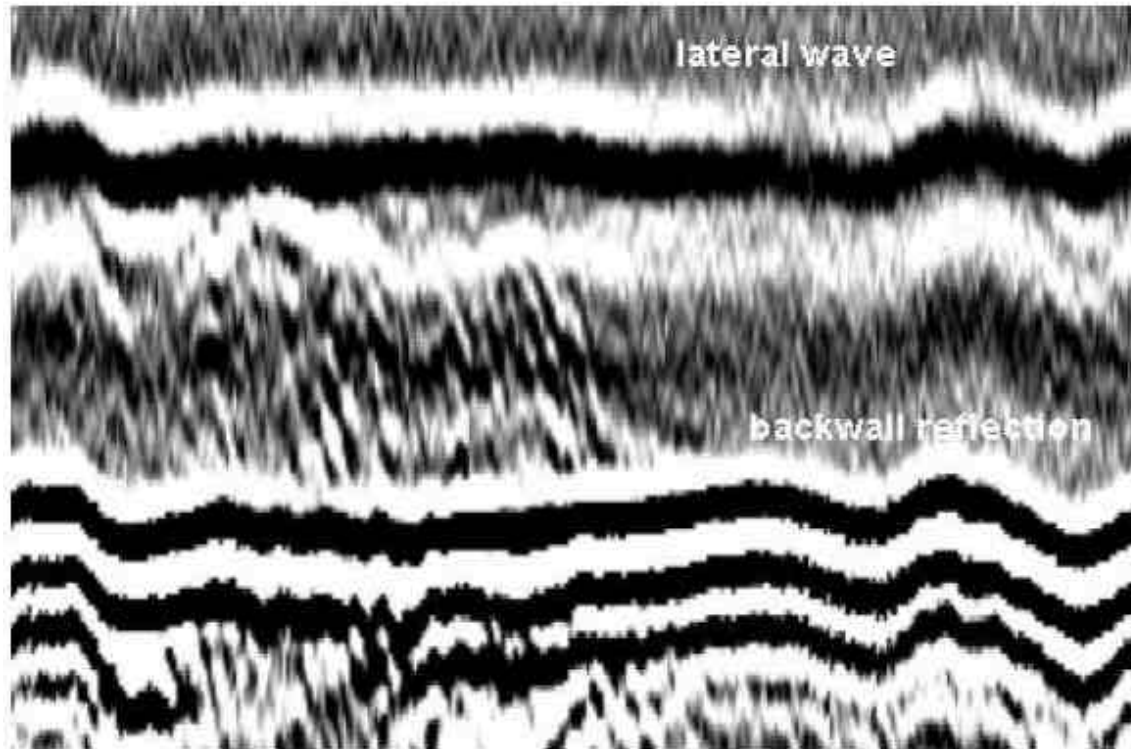
Figure B.3 — Gain setting too high Amplitude of lateral wave \gg 80 % FSH (saturated)
