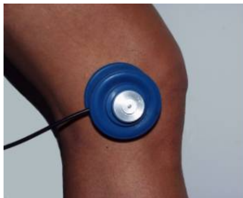
Fig. 4: Position of an acoustic emission sensor at the medial femoral condyle during the measurement
