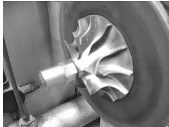
Figure 4: Gas generator compressor impeller.
