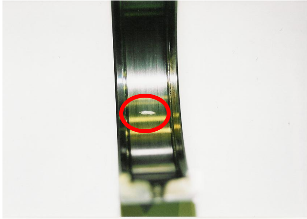
Figure 2 Line defect simulation
