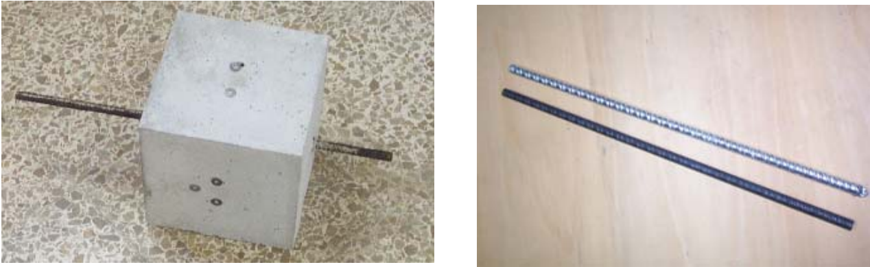
Figure 2: Left: Specimen with bar. Right: Black and galvanized steel bars
