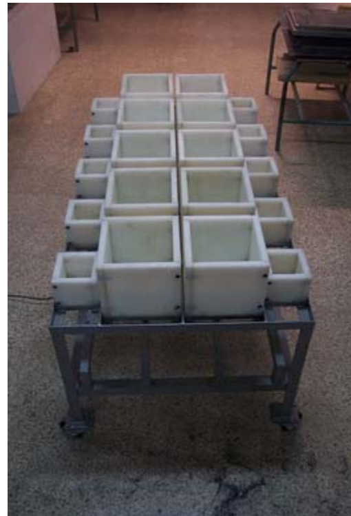
Figure 3: Special table to prepare 20x20x20cm and 10x10x10cm specimens.
