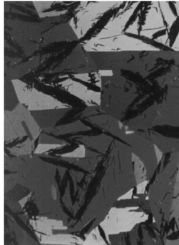
Microstructure of TRIP steel. The so-called martensite disks are black.
