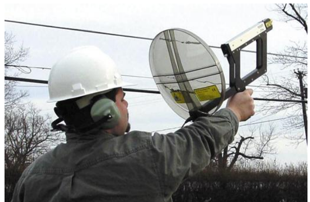
Figure 1: Ultrasound Detector with Parabolic Concentrator
