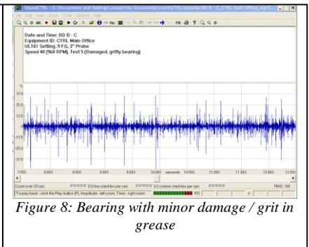
Bearings which are beginning to fail typically have small particles of metal in the lubricant or have small surface irregularity
