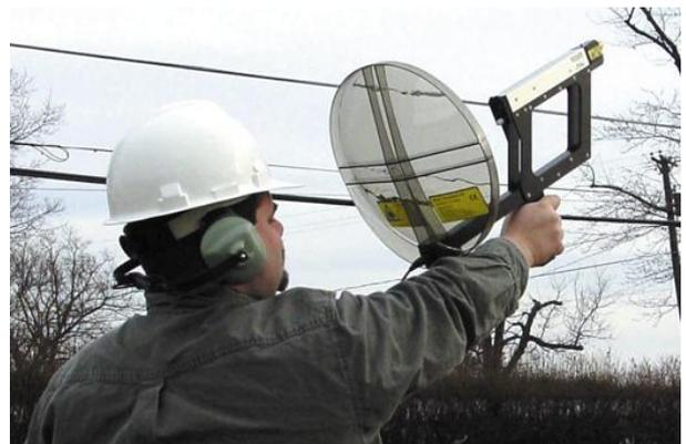
Figure 1: Ultrasound Detector with Parabolic Concentrator
