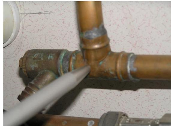
Quite small fluid flows passing through a restriction or bend can produce significant turbulence, generating enough ultrasound to be easily detected. The example illustrated shows the ultrasound levels measured with a contact probe at a joint approximately 30cm from a domestic tap. The smallest stable flow from the tap (approx 0.1 l/minute) produces a signal approximately 15dB higher than the noise level. Signals measured at the tap are far higher
