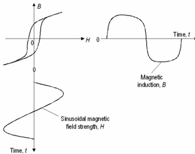
Figure 3: Basics of Nonlinear Harmonic Method.
