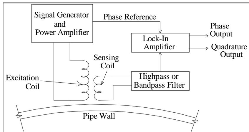
Figure 5: NLH circuit block diagram.
