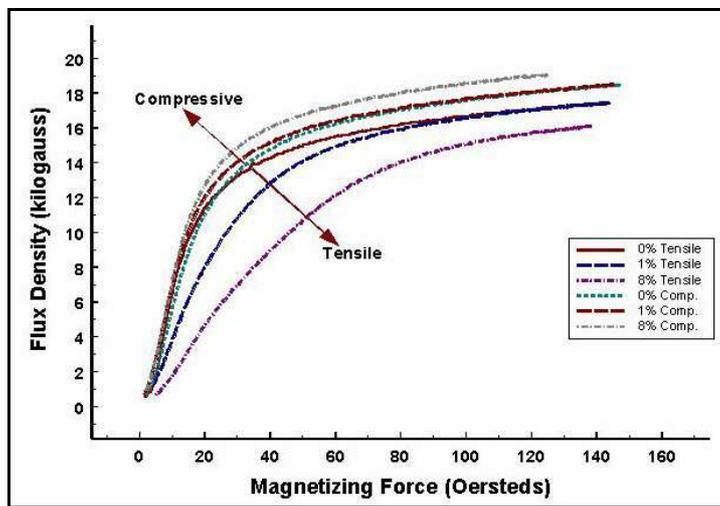
Figure 2: Initial curve and plastic strains.
