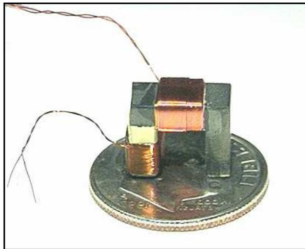
Figure 4: Typical NLH probe.
