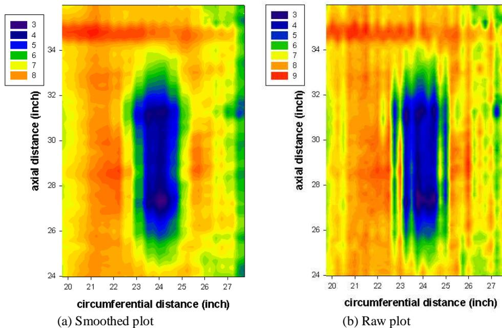
**Figure 9: Blow-up of circumferential field NLH signal results for defect 2-4 comparing a smoothed plot (a) with a plot based on the raw data (b).**
