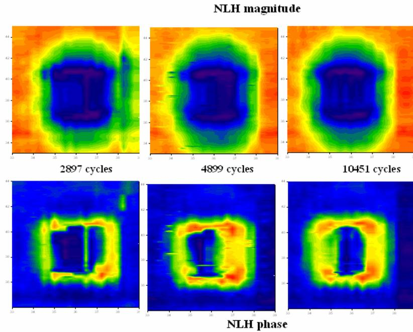
**Figure 11:** From left to right, NLH circumferential magnetic field scan results obtained for defect 2-5 in pipe sample 2 after 2897, 4899 and 10451 pressure cycles. The top figures are the measured NLH magnitudes, and the lower ones the NLH phase angles.
