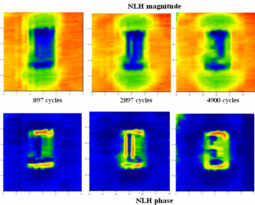
**Figure 12:** From left to right, NLH circumferential magnetic field scan results for defect 5-6 in pipe sample 5 after 897, 2897, and 4900 pressure cycles. The top figures are the measured NLH magnitudes, and the lower ones the NLH phase angles.
