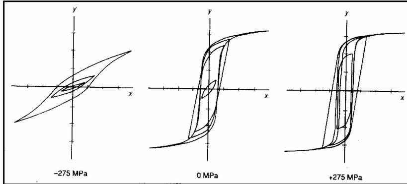
Figure 1: Magnetic properties vary with specimen loading.
