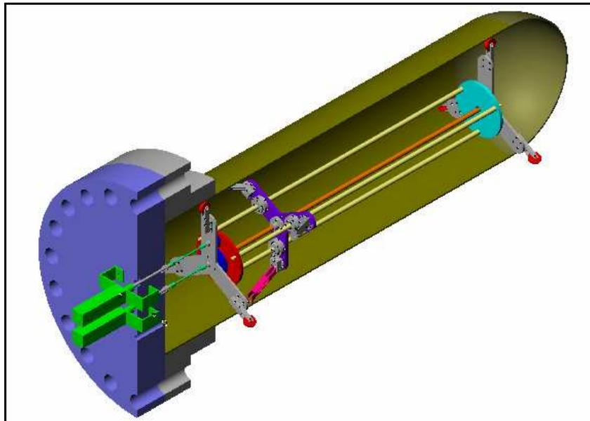
**Figure 6: CADD drawing of internal pipe scanner for NLH during pressure testing.**
