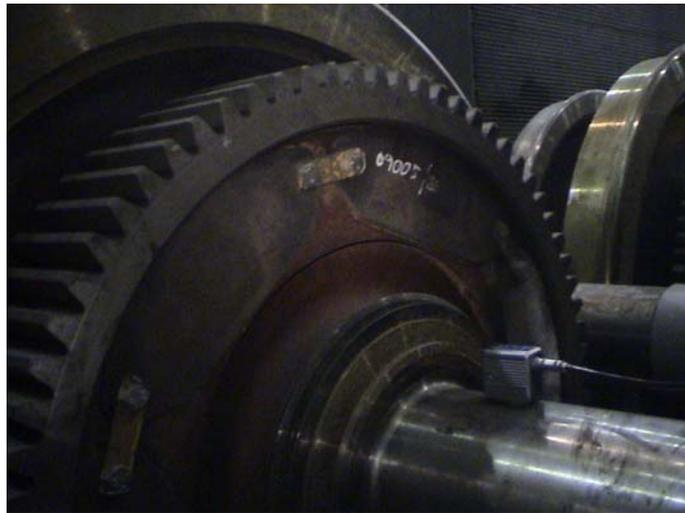
Fig. 5: Ultrasonic inspection with angle probe to confirm a flaw under hub.
