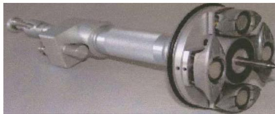
Fig. 14: Probe system for shaft-front testing used at the Italian Railways.
