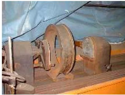
Fig. 1: Magnaflux device for detecting flaws in the material of axles and crankshafts.
