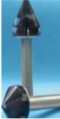
Fig. 16: Kirner probe for testing of shaft studs and axle ASW 29/90.
