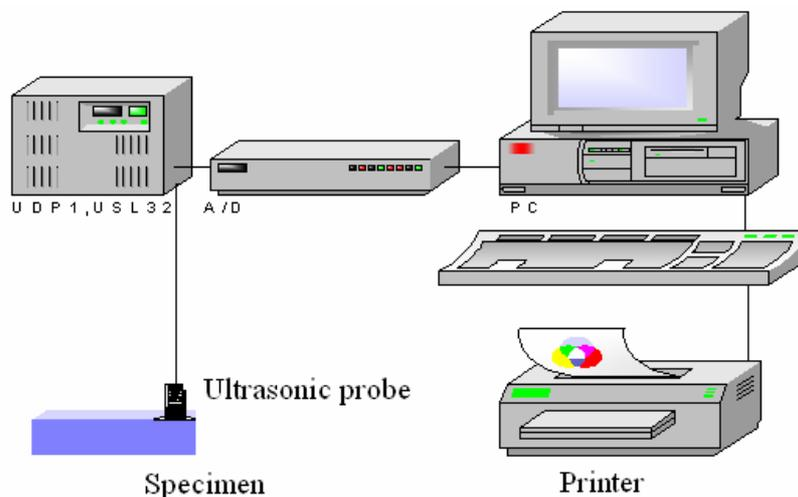
Fig. 6: Experimental system for testing of axles and shafts.
