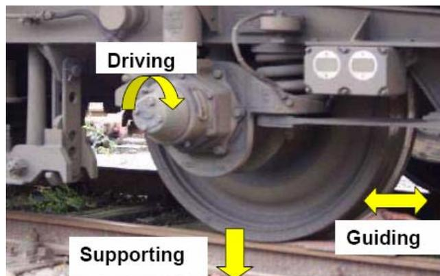
Fig. 2: Bogie with shaft or axle and wheel moving along a rail.
