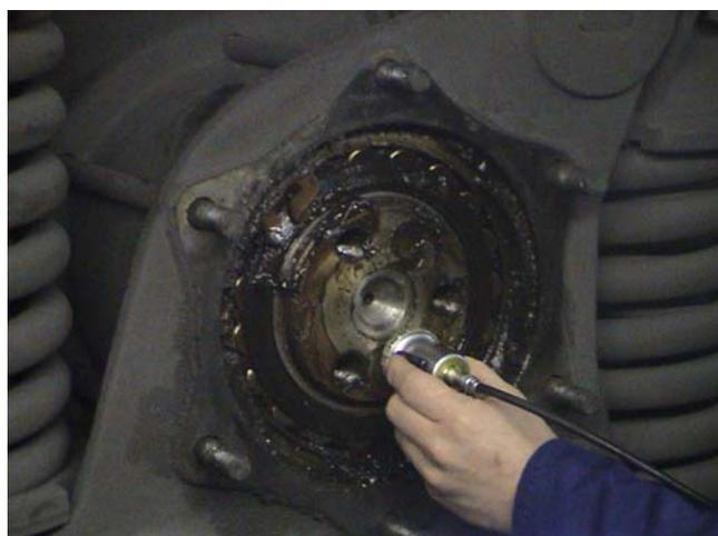
Fig. 4: Ultrasonic inspection from shaft front.
