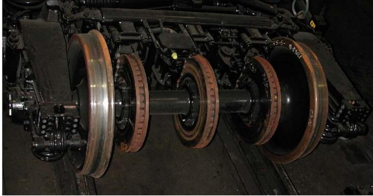
Fig. 20: Inspection of railway shaft using phase transmission.
