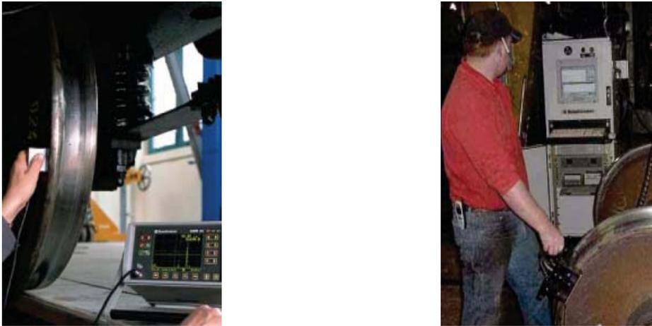
Fig. 18: Left: testing with angle probe; Right: testing with special ultrasonic device.
