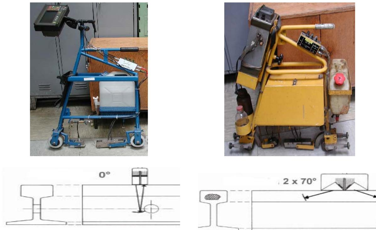
Fig. 19: Rail inspection with single and double ultrasonic probes.
