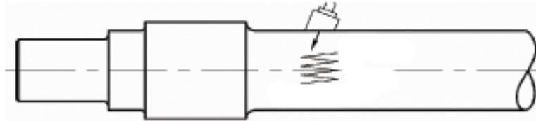
Fig. 3: Testing of axle with AW 37 angle probe.
