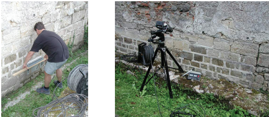
Figure 1. Left: Manual heating of the surface with an infrared radiator. Right: Recording of surface temperature with an infrared camera during cooling down.
