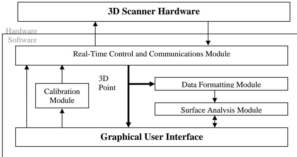
**Figure 3: MILT software block diagram.**
