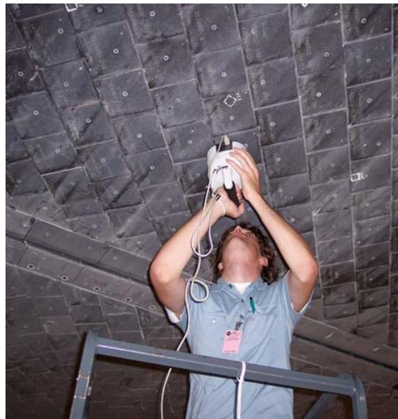
**Figure 5. MILT in use on orbiter Discovery at Kennedy Space Center.**
