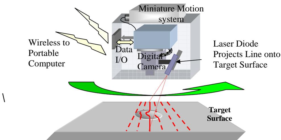
**Figure 1: Model of MILT 3D Scanner architecture**
