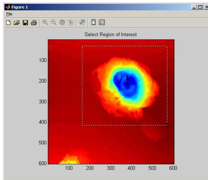
**Figure 6. Flaw detection from MILT scan.**
