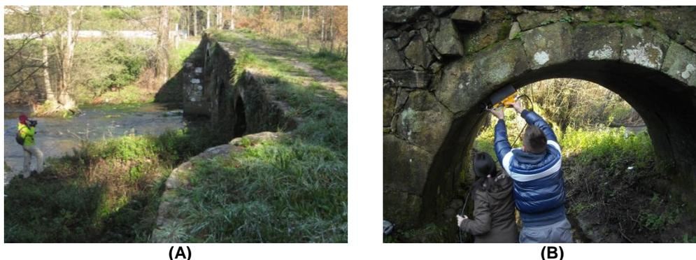
Fig.1. Thermographic survey on the first arch upstream (A) and GPR survey over the vault of the same arch (B)
