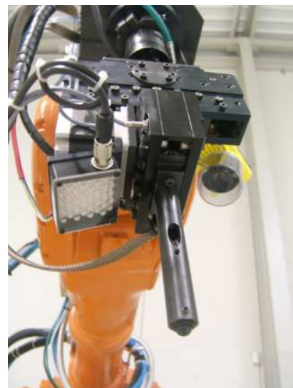
Figure 10: CYCLOPS test head showing machine vision system and probe manipulator
