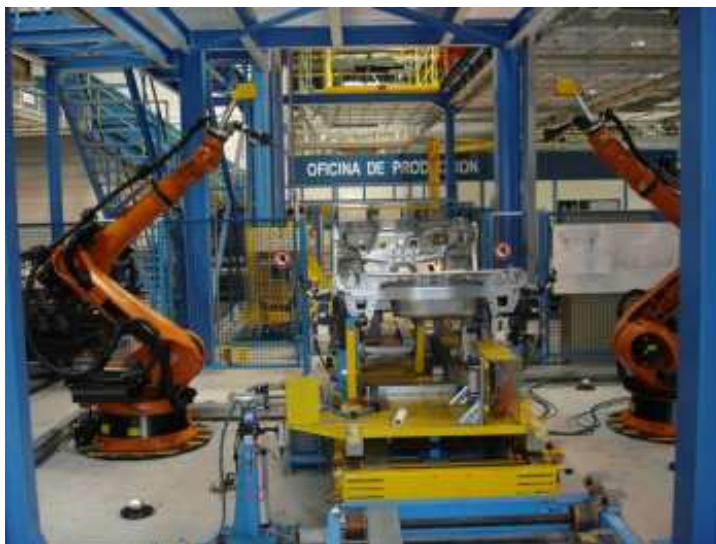
Figure 9: General view of a production CYCLOPS system using dual robotic test heads
