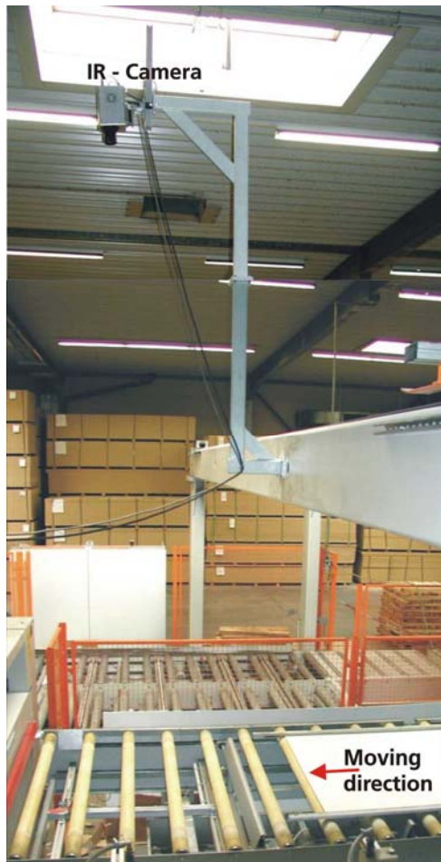
Fig. 3: Thermographic set-up just behind a paper laminating press. By moving the material along the infrared camera possible defects can be detected.
