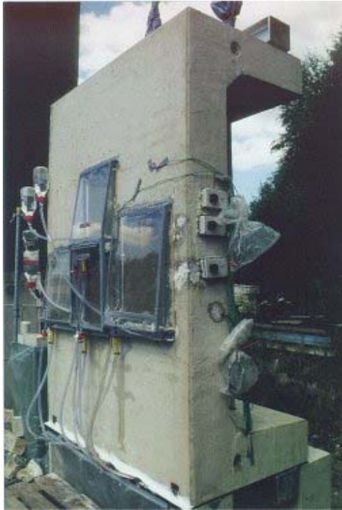
Fig 1a: Left: concrete testing structure with test regions for aggressive solutions
