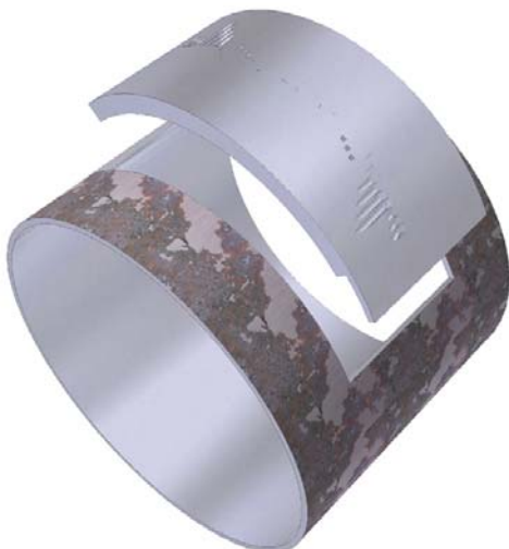
Transducer holders and jigs for custom pipes and flanges are modeled in 3D to fit an exact replica of the item to be inspected.
