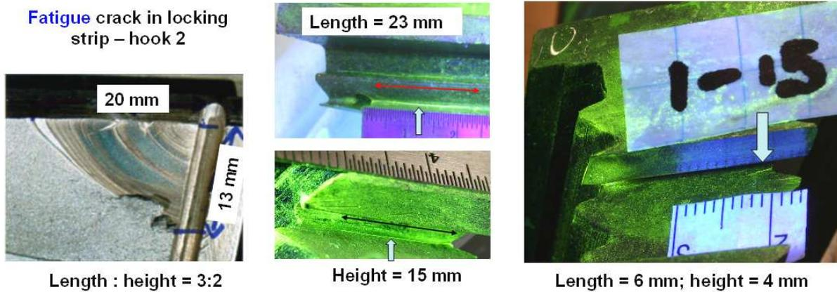
**Figure 4:** Examples of fatigue cracks located in the locking strip area confirmed by MP and fracture mechanics.
