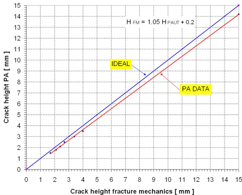
**Figure 11:** PAUT sizing capability compared to fracture mechanics. Crack height range: 1.6 mm – 15 mm. An under-sizing trend between 0.5 mm to 1.0 mm is noticed.
