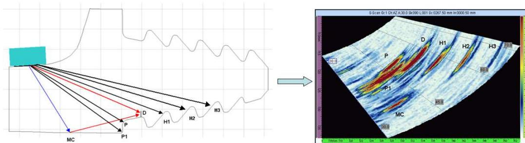
**Figure 13:** Example of crack detection using mode-converted signals.
