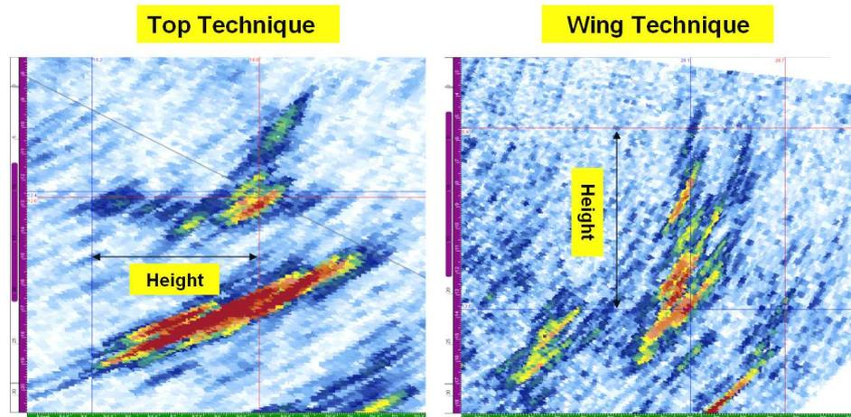
**Figure 7:** Crack sizing method for top and wing techniques.
