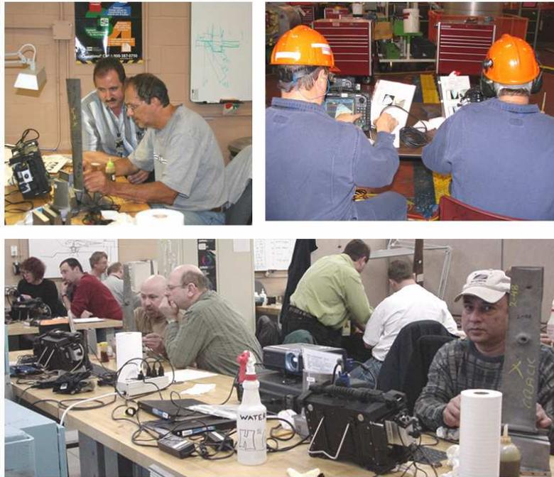
**Figure 8:** Examples of training activities using retired-for-cause blades with cracks and actual PAUT techniques.
