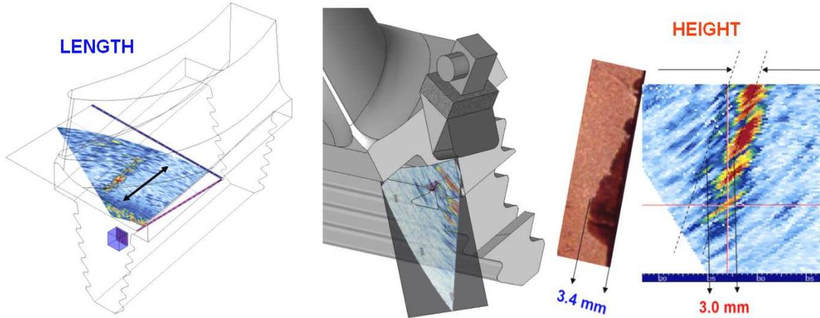
**Figure 6:** Side technique used for confirmation and sizing of SCC and fatigue cracks located in the locking strip-hook 2.
