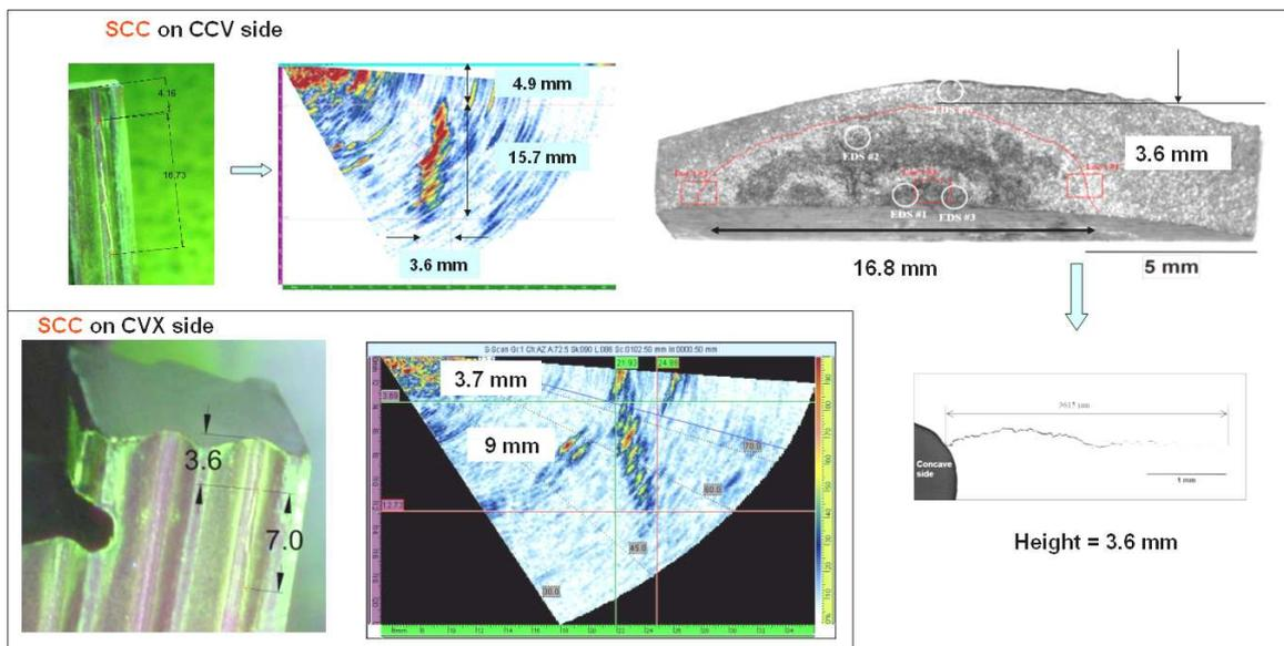
**Figure 12:** Examples of SCC sizing and confirmation by MP, PAUT and fracture mechanics.
