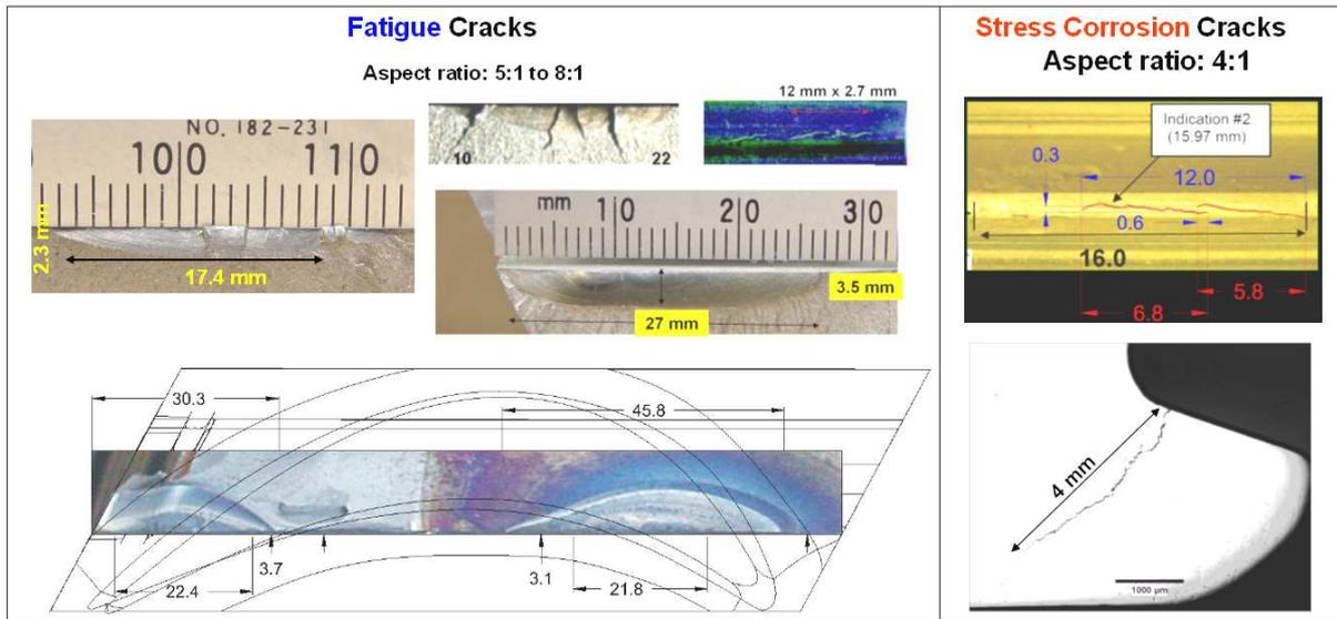
**Figure 3:** Confirmation of fatigue and SCC by fracture mechanics, MP and rubber replica.
