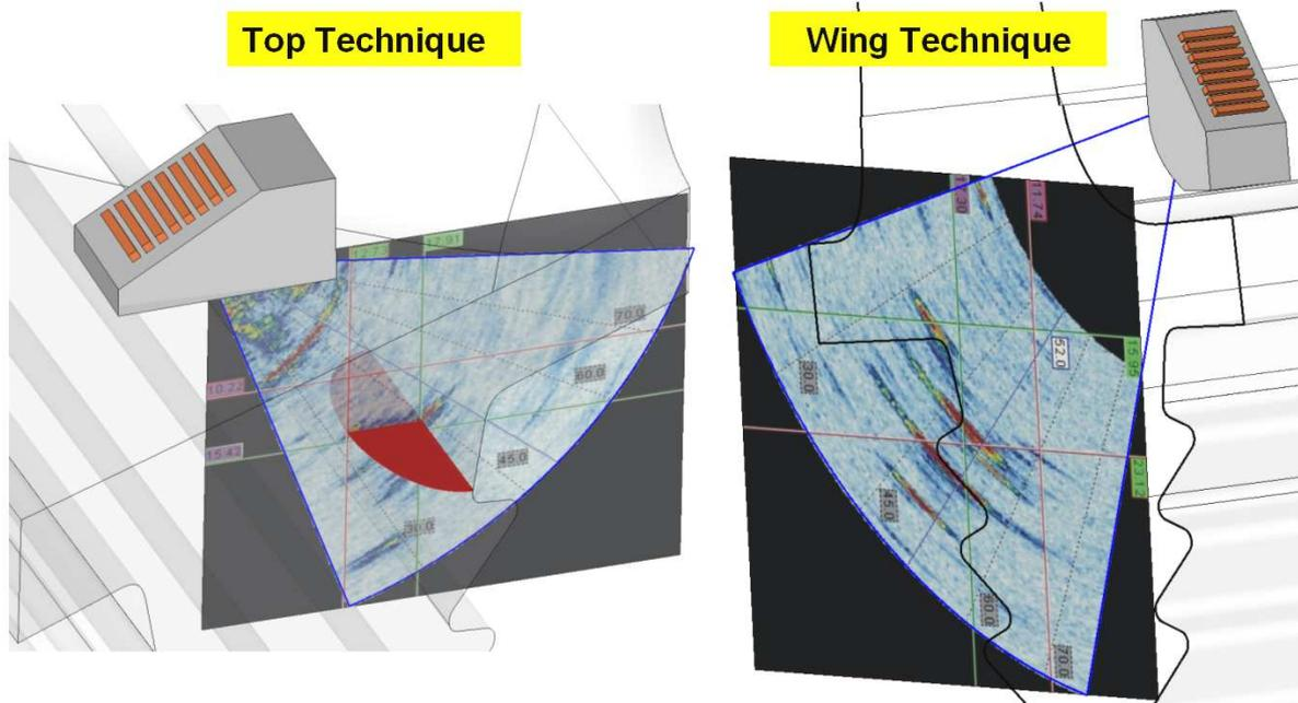
**Figure 5:** Top (*left*) and wing (*right*) techniques used for detection of cracks in Siemens-Parson blades.
