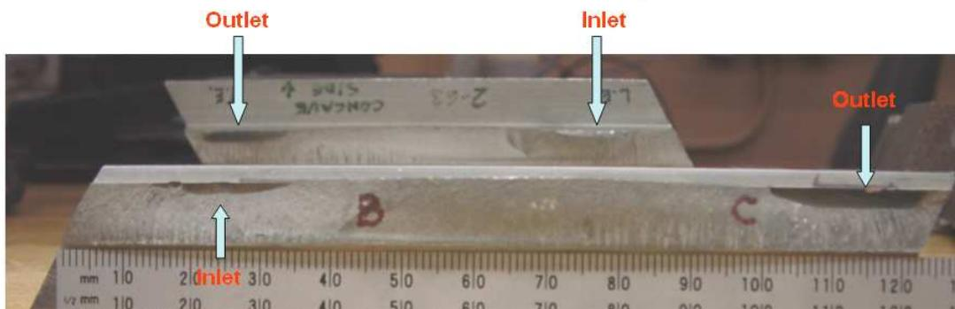
**Figure 2:** Crack locations on concave side confirmed by fracture mechanics on two blades.
