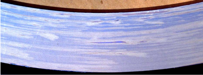
Fig 11: BEA image of distorted surface from friction with non cutting tool material after rework (no anomaly visible before the etch treatment) (prior to rework: see Fig. 3)
