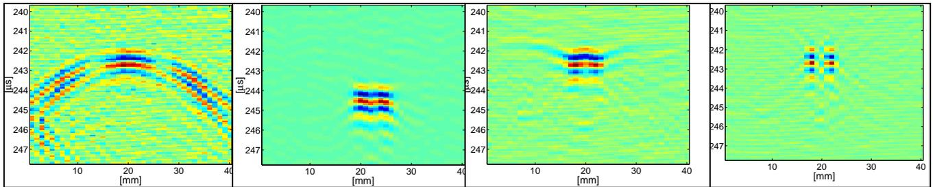
**Figure 7.** B-scans for three compared techniques for SDH distance,  $\Delta d = 5$  mm. From left, respective: original data from 1 mm transducer, PA, SAFT and OLIRB.
