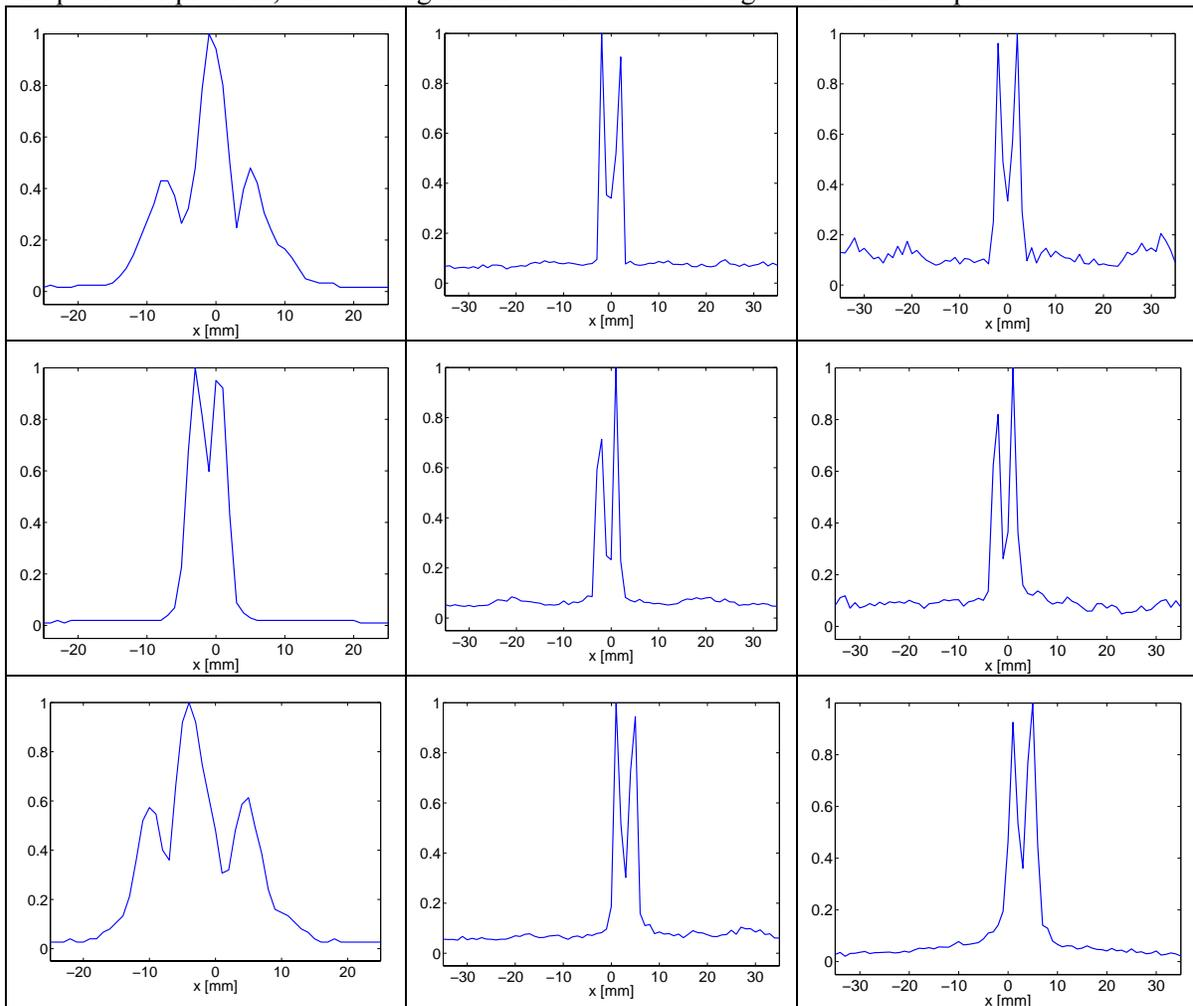
**Figure 4.** Resolution test performed using a pair of steel wires placed 2mm apart in water at three different distances from the array: 60 mm (upper row), 90 mm (middle row) and 120 mm (lower row). Results for a 32 element aperture focused at 60 mm are respectively in the left column, SAFT for single element in the
