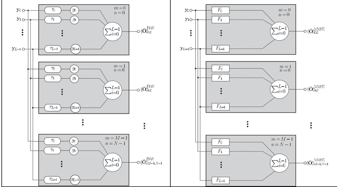
**Figure 1.** Graphical illustration of the operation of parallel DAS (a), and the proposed OLIRB (b).
