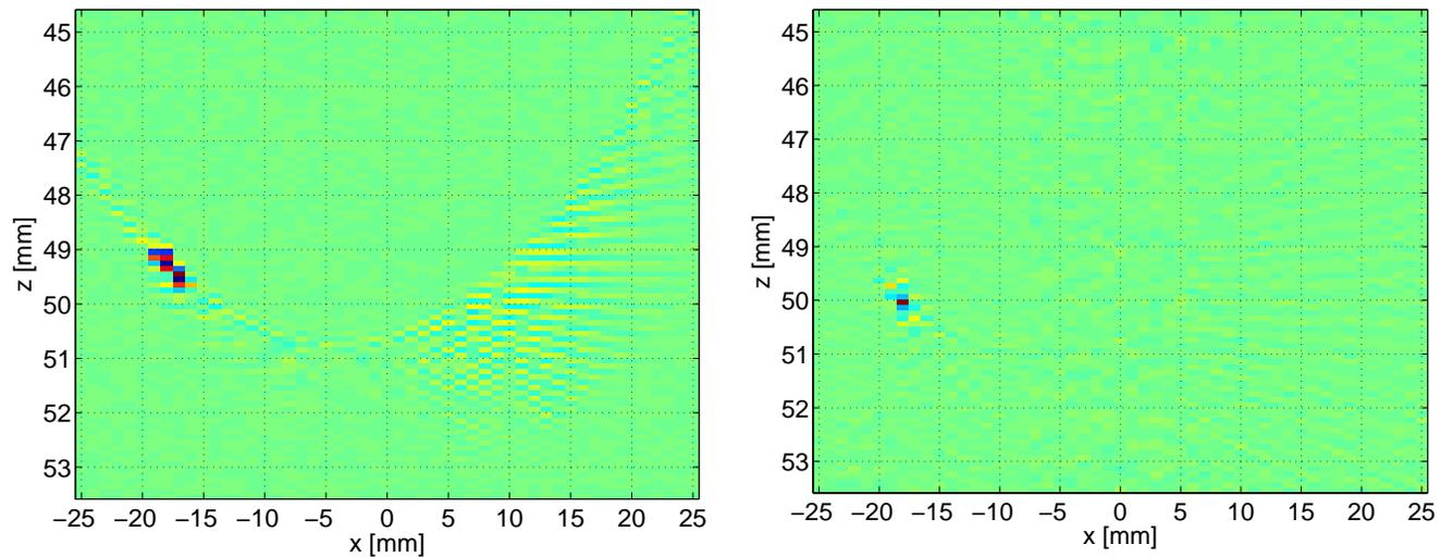
**Figure 3.** Beamformed data obtained for a point target located in the main lobe of a 16 element phased array steered at an angle  $-20^\circ$  and focused at 50 mm. Parallel DAS on simulated data (left) and OLIRB on simulated data (right).
