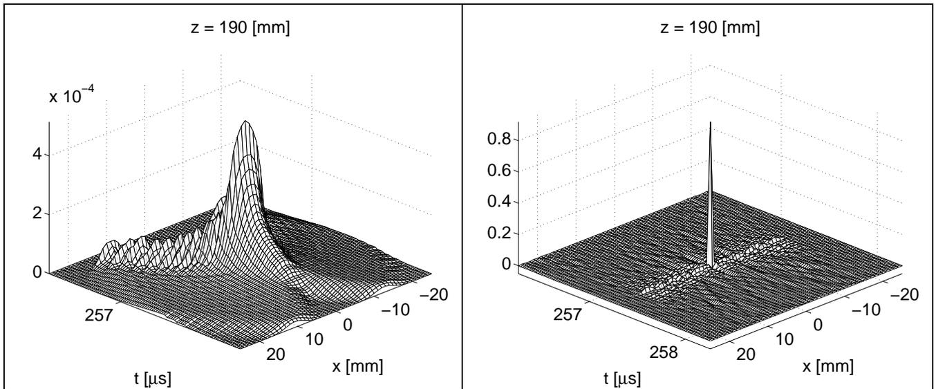
**Figure 2.** Simulated B-scans obtained for 8 mm transducer processed with SAFT (left) and ESAFT (right).
