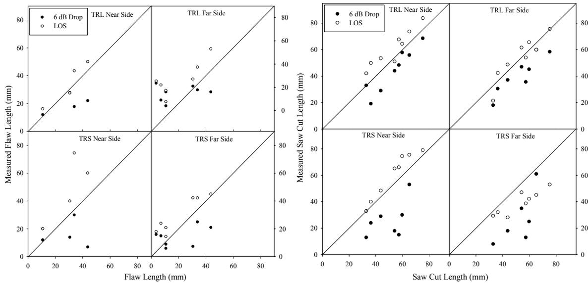
**Figure 4** - Length-sizing data for saw cuts and implanted flaws using 6dB drop and LOS methods.
