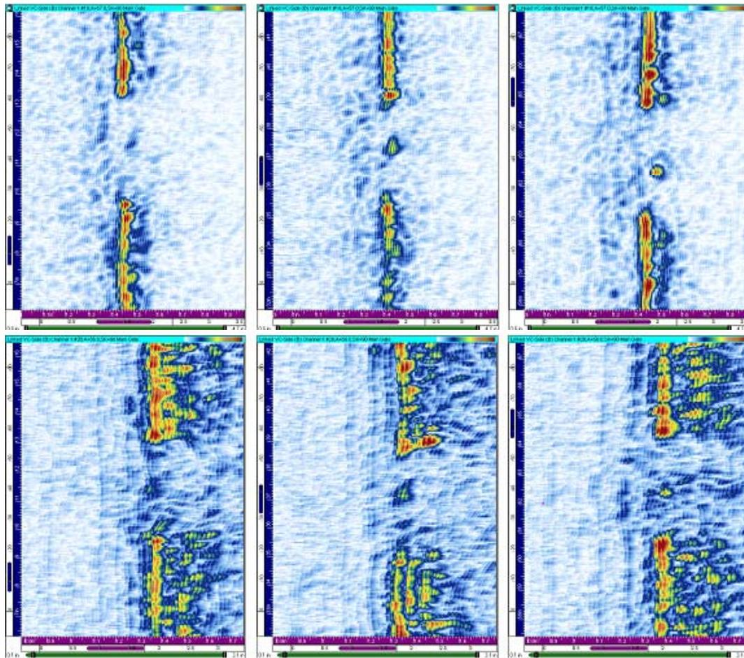
**Figure 8** - B-Scan views for ultrasonic responses from three implanted flaws (left-to-right: 5, 10 and 15% through-wall cracks) in weld two from the far-side with the TRS (top) and TRL (bottom) arrays.
