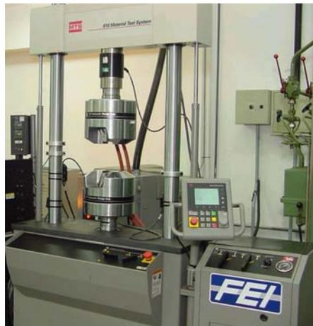
Illustration 5. MatLab-FEI's universal testing machine MTS
