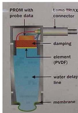
Illustration 2. Schematic representation of the used transducer.
