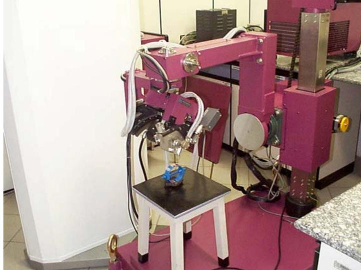
Illustration 3. Rigaku MSF-3M diffractometer X-Ray Analyser
