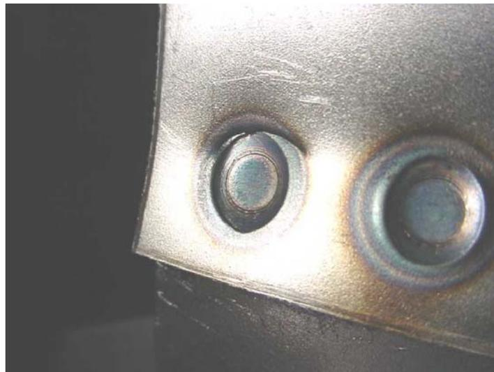
Illustration 9: Experimental proof of crack appearance in von Mises maximum stress area.
