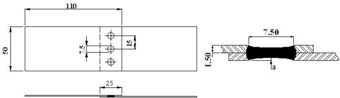
Illustration 1. Welded specimen in study and spot weld geometry.
