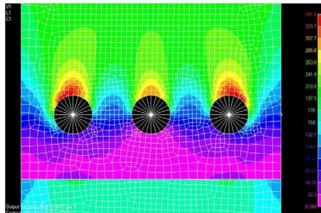
Illustration 6: Results of the simulation through FEM for the maximum principal stress ( $\sigma_{\max PR} = \sigma_{\text{medPR}} + \Delta\sigma_{PR}$ ) with plate elements, showing stress concentration area in the most external spots.
