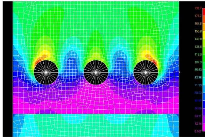
Illustration 7: Results of the simulation through FEM for the von Mises stress with plate elements, showing area of  $\sigma_{med}$  concentration in the most external spots.
