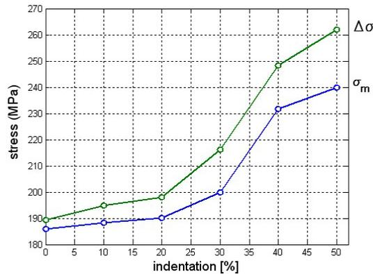
Illustration 8: Maximum main stress components variation in function of spot weld indentation. Results of the simulation through FEM with solid elements.
