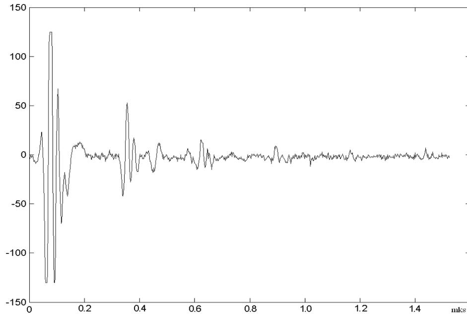
Figure 1 Typical A-scan obtained from 0.7 mm steel-0.3 mm epoxy structural adhesive- 0.7 mm steel structure
