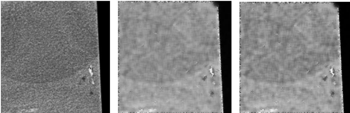
Figure 3. Result of filtering. a) application of low-pass filter to each A- scan; b) spatial filtering of the image; c) combination of the both procedures.
