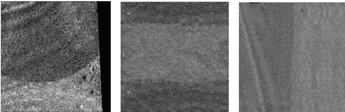
Figure 4 Result of cross-correlation processing of acoustical data. a) boundary adhesive-lack of adhesive; b) strip of Teflon spray on the interface; c) boundary uncured-cured adhesive
