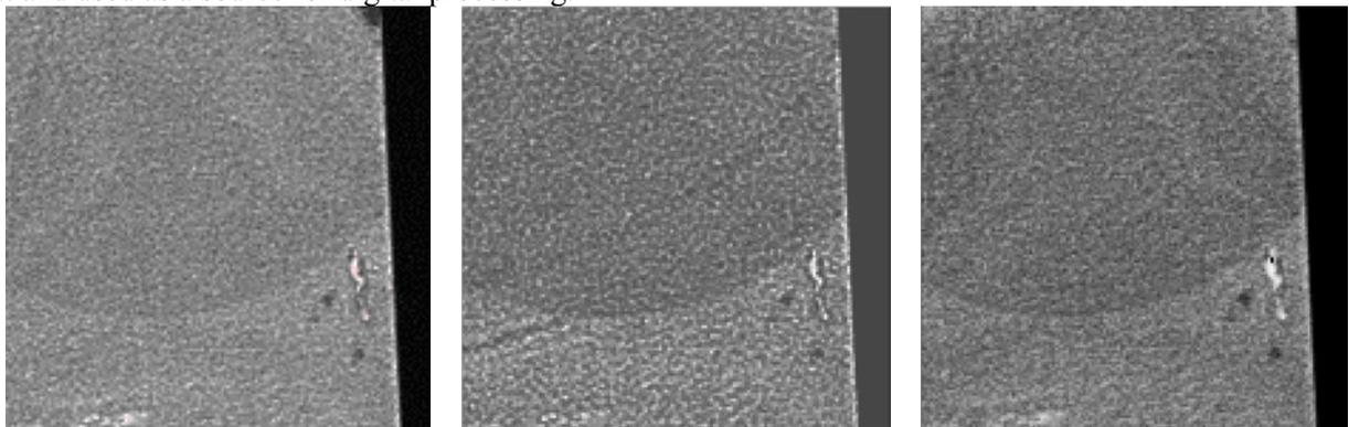
Figure 2. a) C-scan of the steel-epoxy interface (area 20 x 20 mm); b) multiplication of C-scans ,corresponding to several reflections; c) image representing attenuation coefficient distribution
